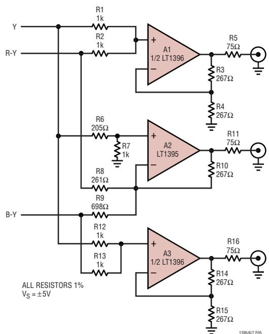
Figure 5. Buffered Color-Difference to RGB Matrix
