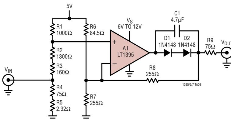
Figure 6. Single Supply RGB Video Amplifier (1 of 4 Channels)
