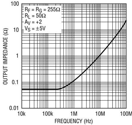
**LT1395CS6 Output Impedance (Disabled) vs Frequency**
