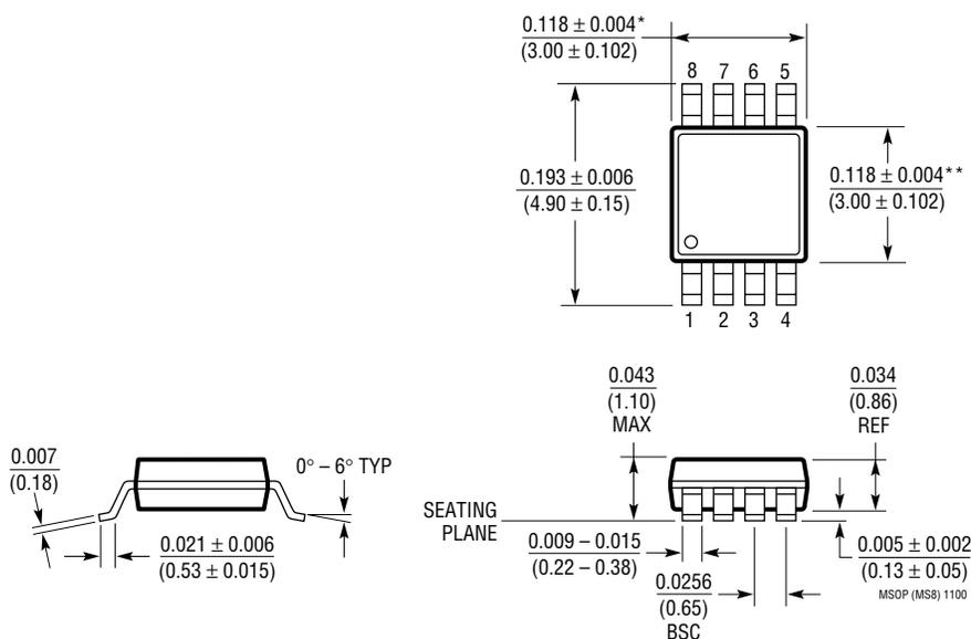
\* DIMENSION DOES NOT INCLUDE MOLD FLASH, PROTRUSIONS OR GATE BURRS. MOLD FLASH, PROTRUSIONS OR GATE BURRS SHALL NOT EXCEED 0.006" (0.152mm) PER SIDE
