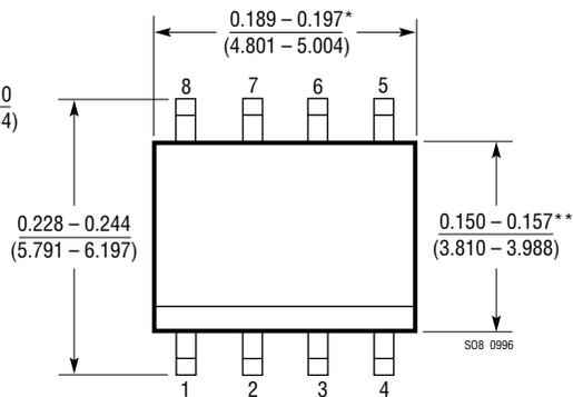
\*DIMENSION DOES NOT INCLUDE MOLD FLASH. MOLD FLASH SHALL NOT EXCEED 0.006" (0.152mm) PER SIDE
