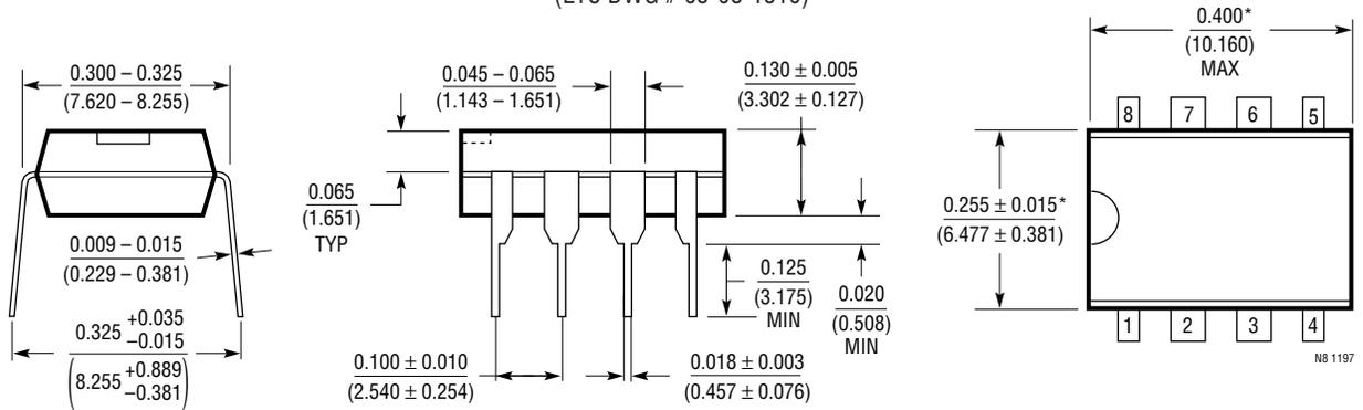
\*THESE DIMENSIONS DO NOT INCLUDE MOLD FLASH OR PROTRUSIONS.
