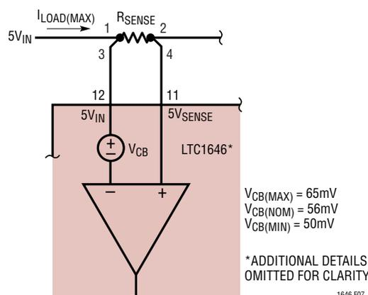
Figure 7. Circuit Breaker Equivalent Circuit for Calculating  $R_{SENSE}$
