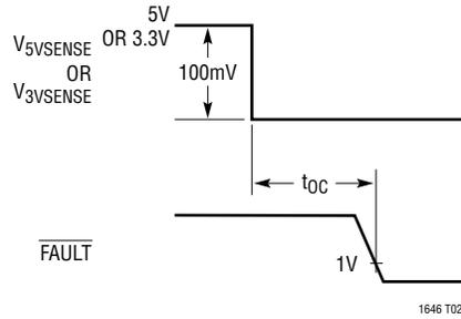
**t<sub>SC</sub> Short-Circuit Fault Detect**
