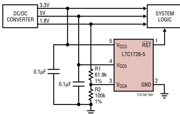
**Triple Supply Monitor with Power Good Output (3.3V, 2.5V and Adjustable)**
