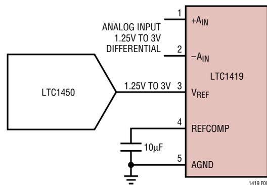
Figure 9. Driving V<sub>REF</sub> with a DAC
