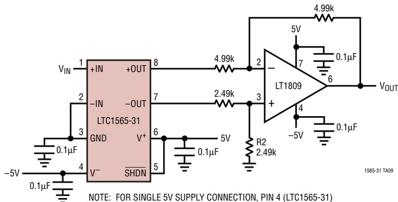
NOTE: FOR SINGLE 5V SUPPLY CONNECTION, PIN 4 (LTC1565-31) AND PIN 4 (LT1809) SHOULD BE GROUNDED AND RESISTOR R2 SHOULD BE DC BIASED AT APPROXIMATELY 2.5V (SEE TEST CIRCUIT FOR SINGLE SUPPLY OPERATION)
