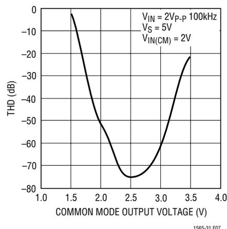
Figure 7. THD vs Common Mode Output Voltage
