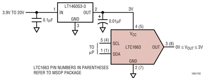
Figure 2. LT1460 As Power Supply for the LTC1663
