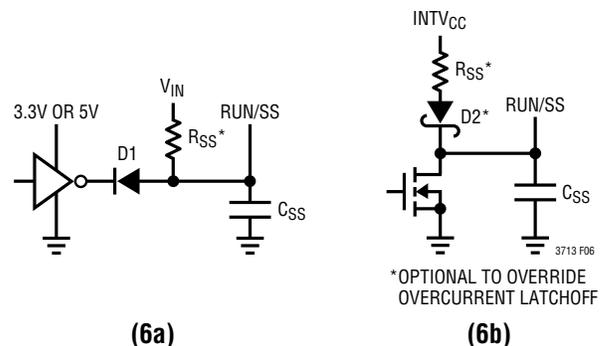
Figure 6. RUN/SS Pin Interfacing with Latchoff Defeated
