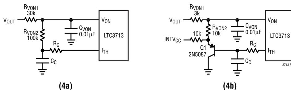
Figure 4. Adjusting Frequency Shift with Load Current Changes
