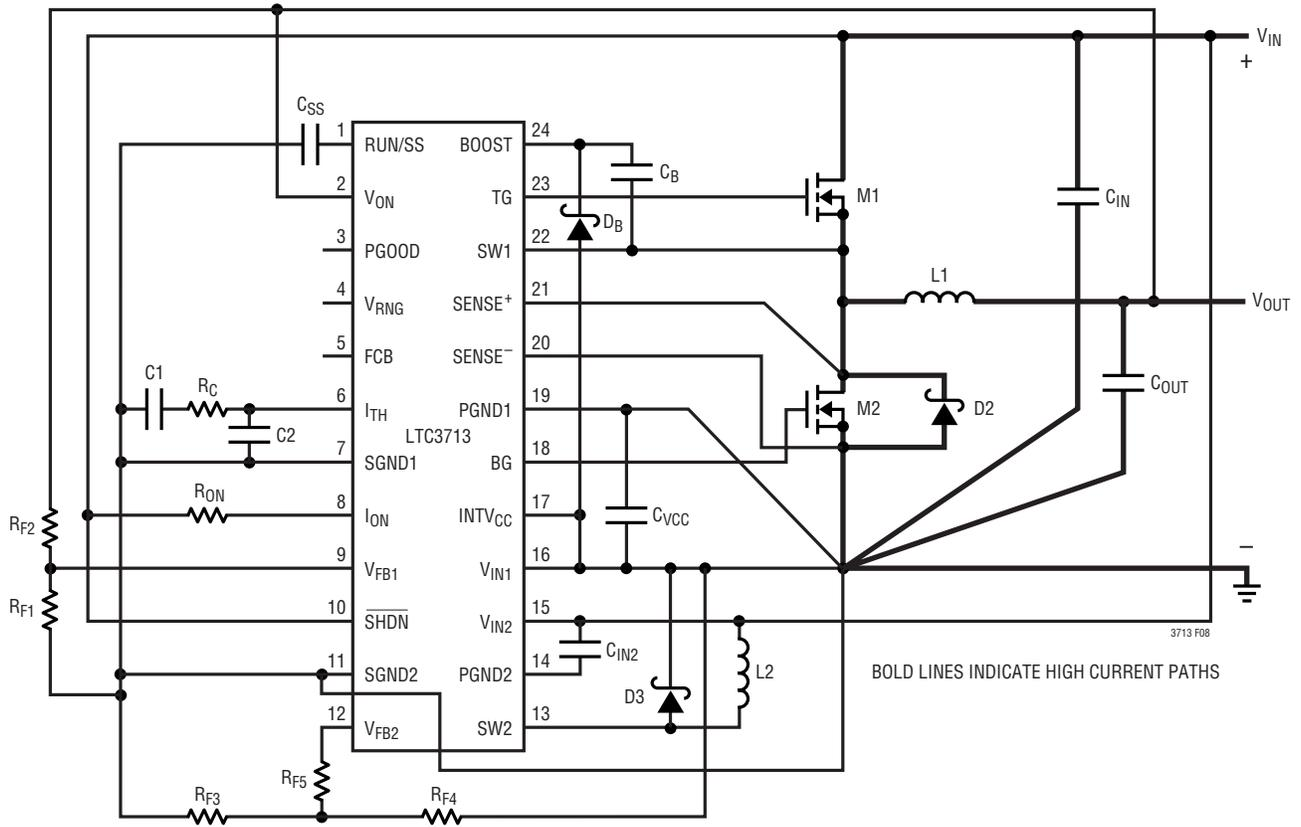
Figure 8. LTC3713 Layout Diagram
