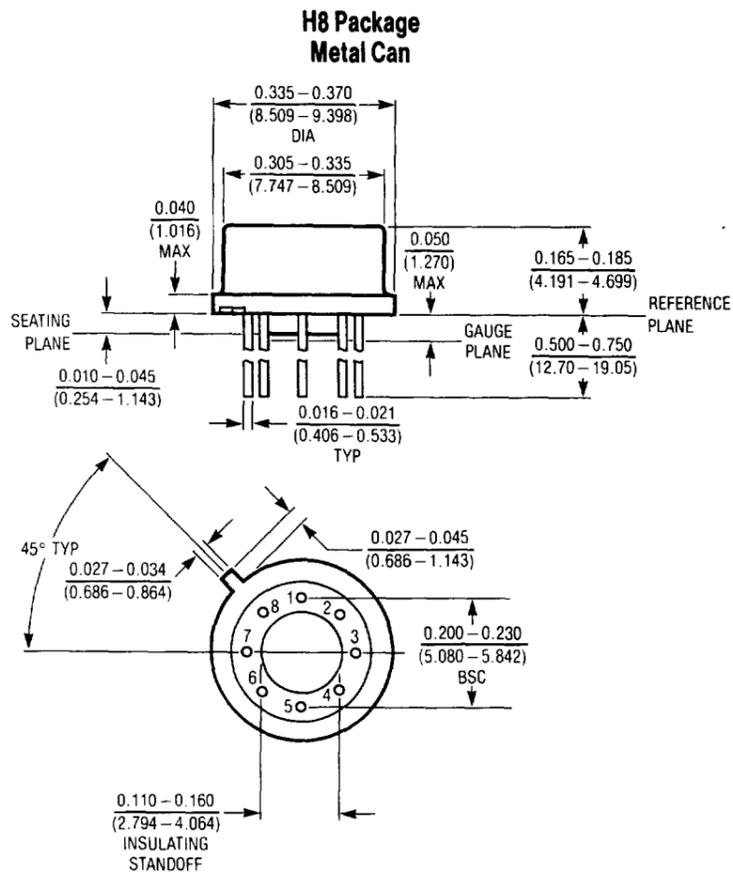
NOTE: LEAD DIAMETER IS UNCONTROLLED BETWEEN THE REFERENCE PLANE AND SEATING PLANE.
