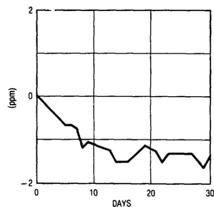
LONG TERM STABILITY OF A TYPICAL DEVICE FROM TIME = 0
