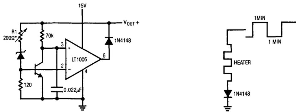
\*PULSE HEATER ON AND OFF TO HEAT AND COOL THE REFERENCE. ADJUST R1 FOR MINIMUM VOLTAGE CHANGE THROUGH A TEMPERATURE CYCLE.
