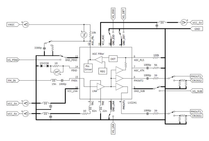
Electrical characteristic in this datasheet is measured by this application circuit. A voltage gain is 9.8dB at 100MHz. The Input/Output impedance is  $50\Omega$ .
