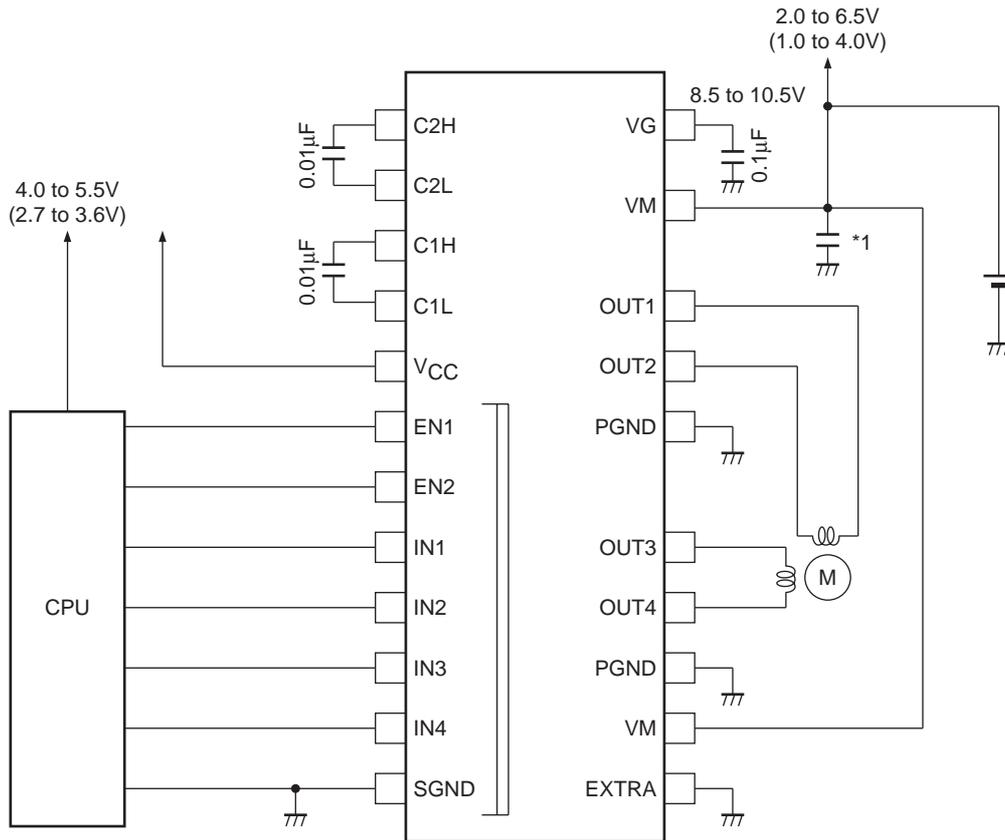
\*1 : Connect a kickback absorption capacitor directly near IC. Coil kickback may cause rise of the voltage of VM line, and the voltage exceeding the maximum rating may be applied momentarily, resulting in deterioration or damage of IC.
