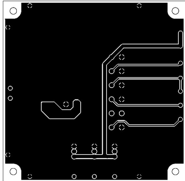
**L2 : Copper wiring pattern diagram**
