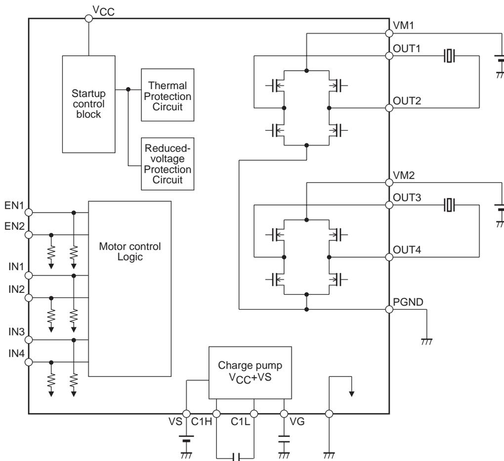
\* Connect a kickback absorption capacitor as near as possible to the IC. Coil kickback may cause increase in VM line voltage, and a voltage exceeding the maximum rating may be applied momentarily to the IC, which results in deterioration or damage of the IC
