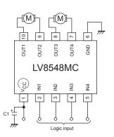
2. Example of applied circuit when one stepping motor driving
