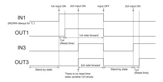
3. Example of current wave type in each excitation mode when stepping motor parallel input is controlled.
