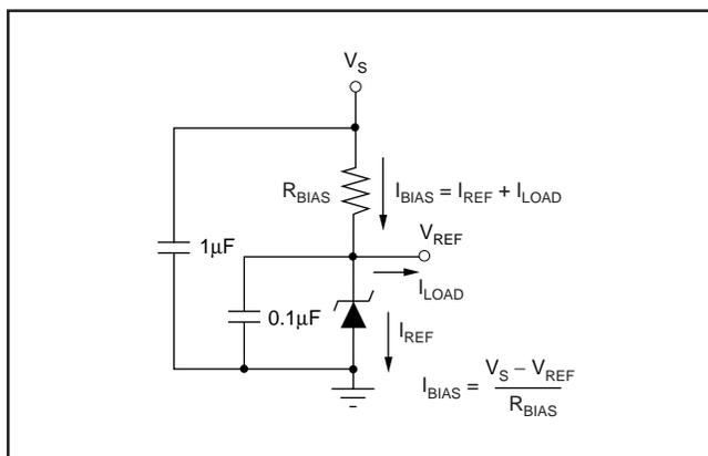
FIGURE 1. Typical Connections.
