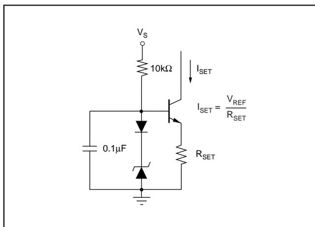
FIGURE 2. REF1112 Provides a Stable Current Source.
