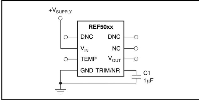
**Figure 25. Noise Reduction Using the TRIM/NR Pin**
