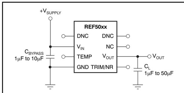
Figure 23. Basic Connections
