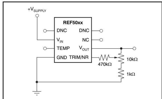
Figure 24.  $V_{OUT}$  Adjustment Using the TRIM/NR Pin
