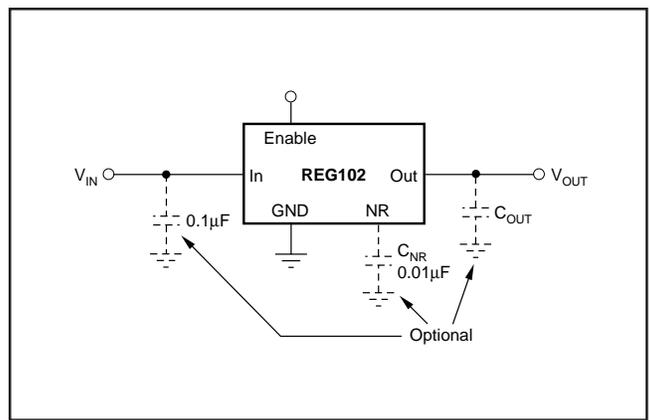
FIGURE 1. Fixed Voltage Nominal Circuit for the REG102.
