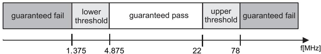
Figure 4-8. LPO and Clock Detection, Untrimmed CLK10M
