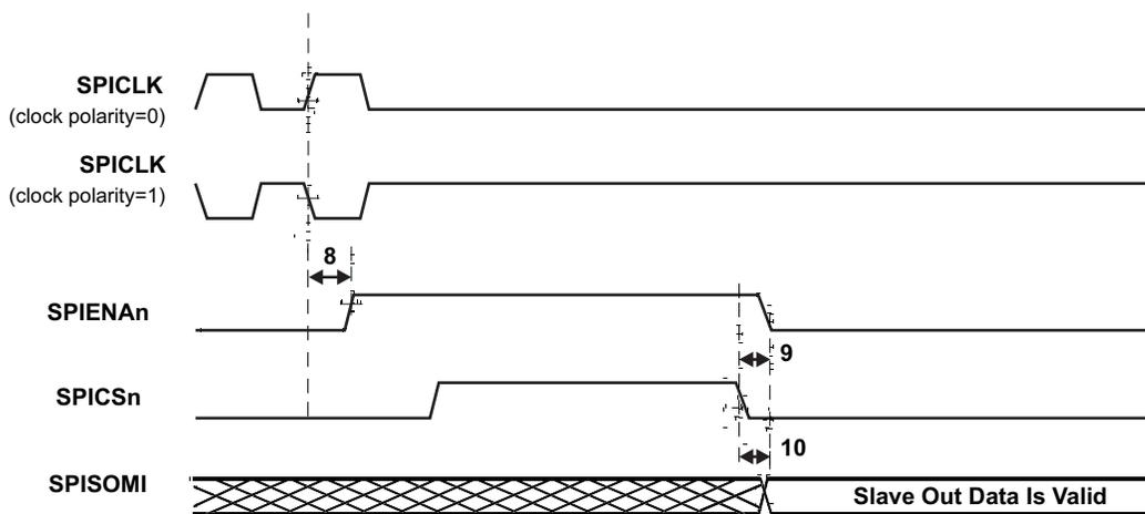
Figure 5-13. SPI Slave Mode Enable Timing (CLOCK PHASE = 1)
