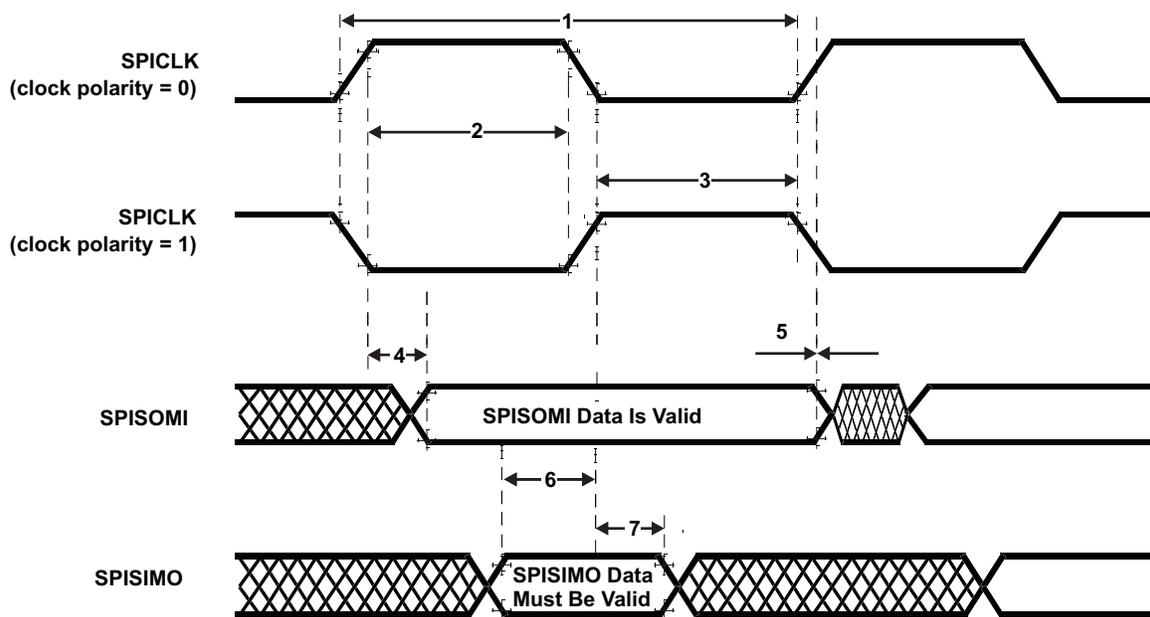
Figure 5-10. SPI Slave Mode External Timing (CLOCK PHASE = 0)
