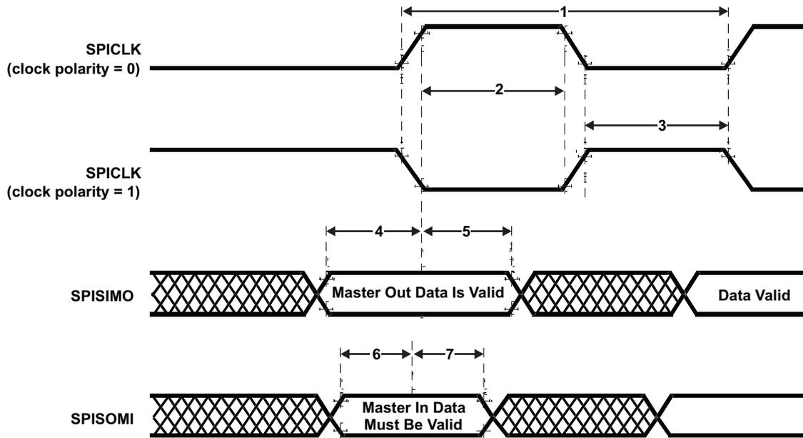
Figure 5-8. SPI Master Mode External Timing (CLOCK PHASE = 1)
