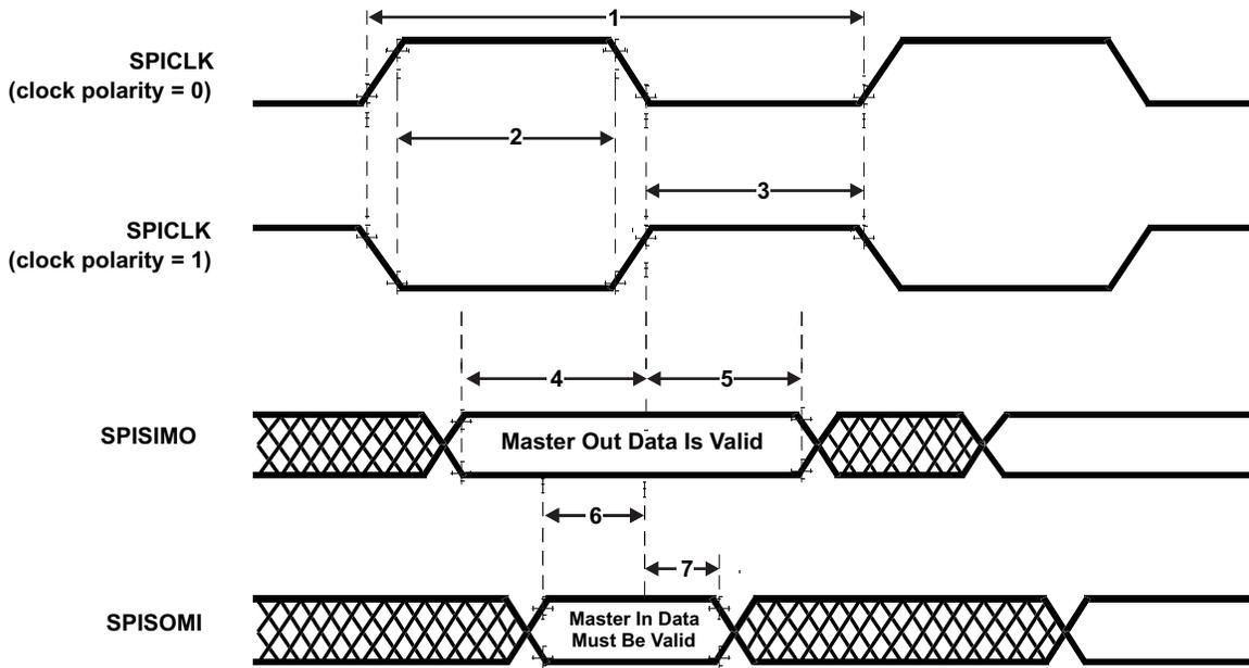
Figure 5-6. SPI Master Mode External Timing (CLOCK PHASE = 0)
