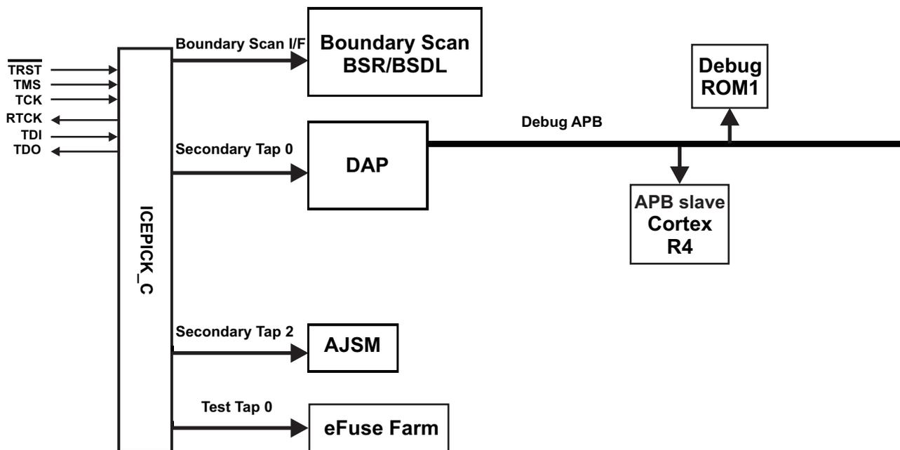
Figure 4-13. ZWT Debug Subsystem Block Diagram
