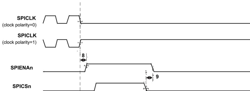
Figure 5-11. SPI Slave Mode Enable Timing (CLOCK PHASE = 0)
