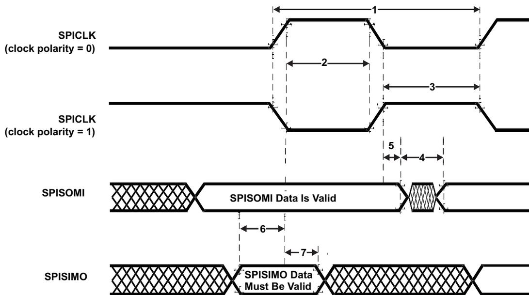
Figure 5-12. SPI Slave Mode External Timing (CLOCK PHASE = 1)
