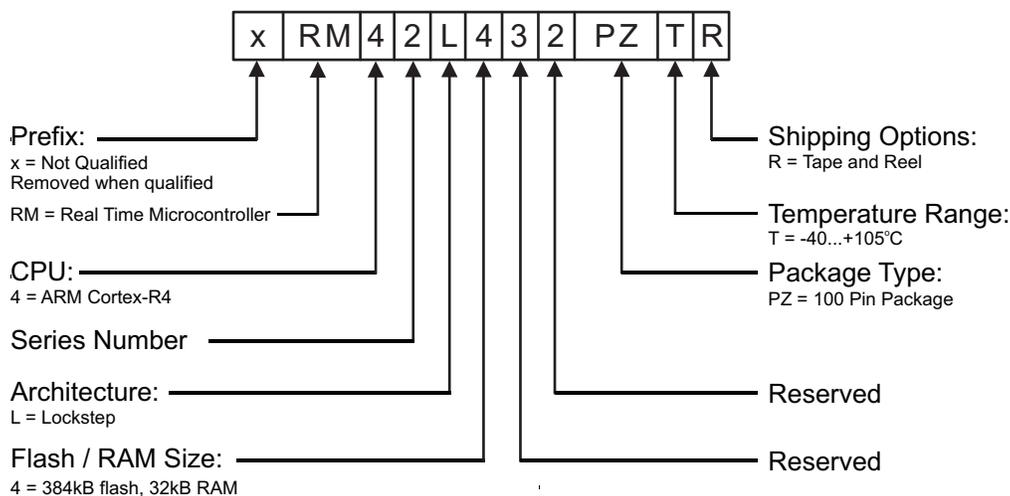
Figure 6-1. Device Numbering Conventions
