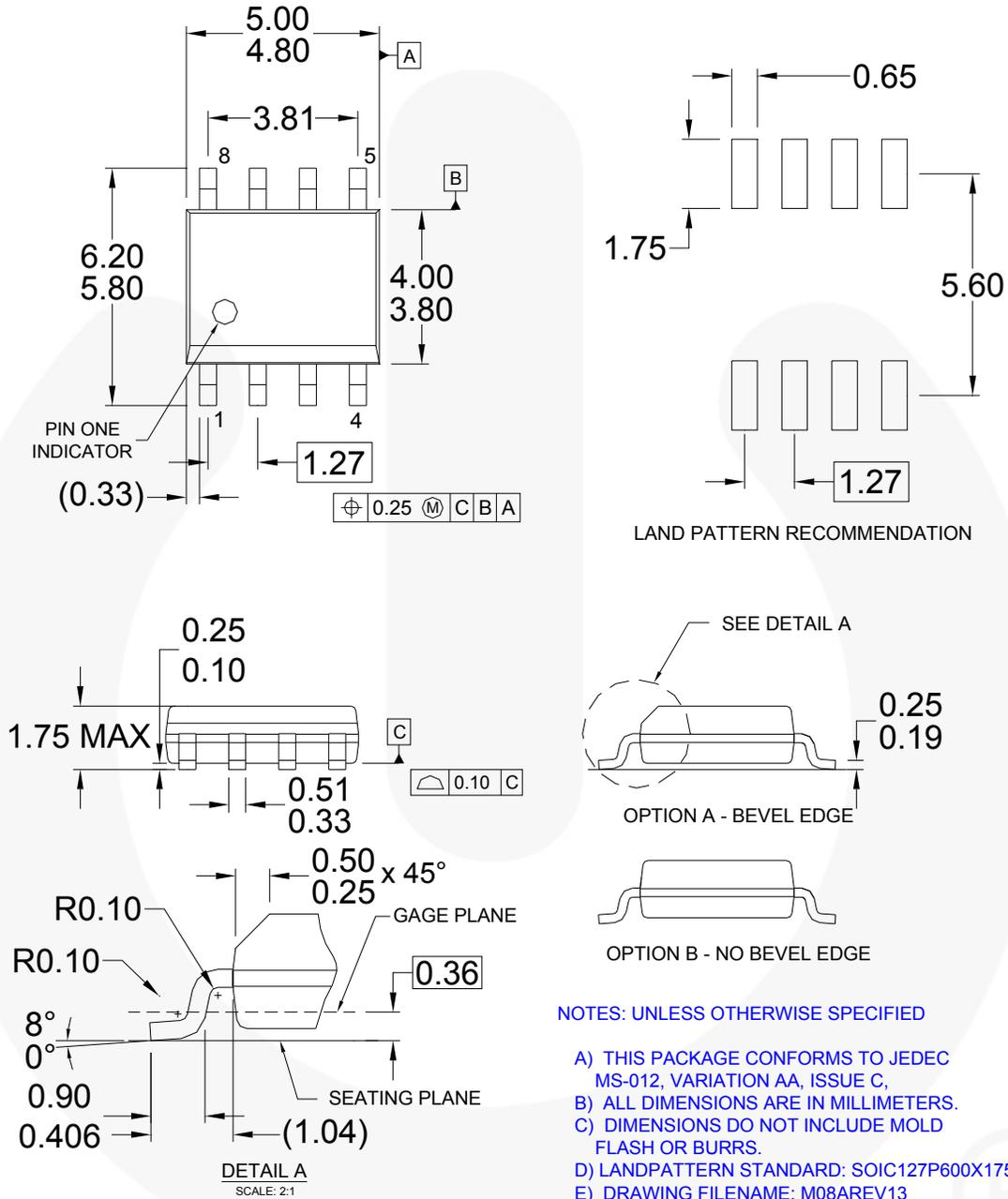
Figure 5. 8-Lead, Plastic Small-Outline Integrated Circuit (SOIC)
