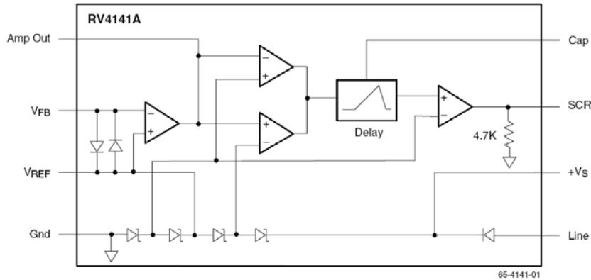
Figure 1. Block Diagram
