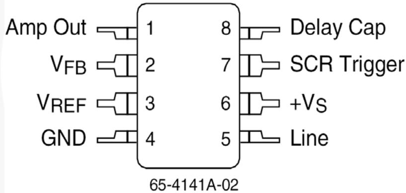
Figure 2. Pin Assignment
