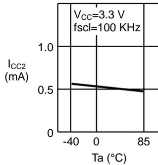
1.11 Current consumption (PROGRAM)  $I_{CC2}$  — Ambient temperature  $T_a$
