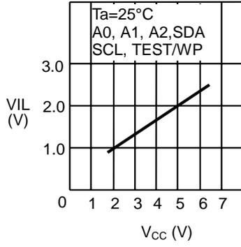
1.26 Low input inversion voltage  $V_{IL}$  —
