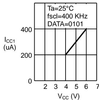
1.7 Current consumption (READ)  $I_{CC1}$  — Clock frequency  $fscl$
