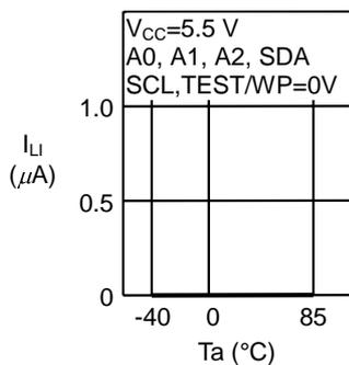
1.16 Input leakage current  $I_{LI}$  — Ambient temperature  $T_a$
