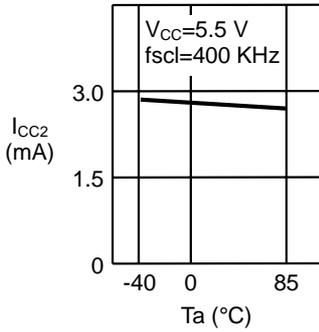
1.10 Current consumption (PROGRAM)  $I_{CC2}$  — Ambient temperature  $T_a$
