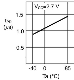
2.7 SDA output delay time  $t_{PD}$  —
