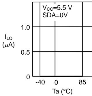
1.18 Output leakage current  $I_{LO}$  — Ambient temperature  $T_a$
