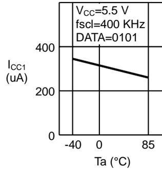
1.3 Current consumption (READ)  $I_{CC1}$  — Ambient temperature  $T_a$
