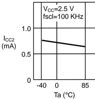
1.12 Current consumption (PROGRAM)  $I_{CC2}$  — Power supply voltage  $V_{CC}$
