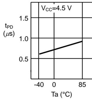
2.6 SDA output delay time  $t_{PD}$  —
