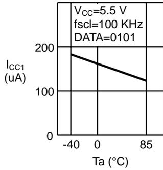
1.2 Current consumption (READ)  $I_{CC1}$  — Ambient temperature  $T_a$
