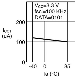
1.4 Current consumption (READ)  $I_{CC1}$  — Ambient temperature  $T_a$
