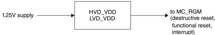
**Figure 5-1. Logic scheme of the core voltage detectors**
