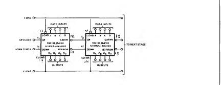
Circuitry is provided internally for cascading these counters. The mode of cascading shown is ripple borrow/carry. No external components are required.
