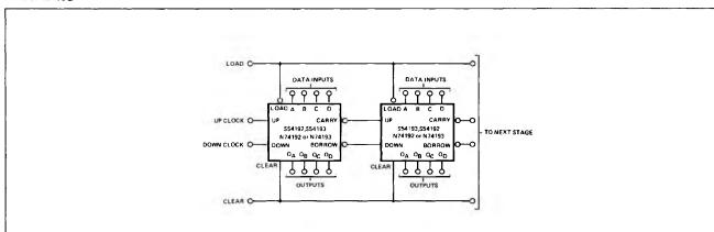
Circuitry is provided internally for cascading these counters. The mode of cascading shown is ripple borrow/carry. No external components are required.
