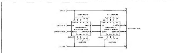
Circuitry is provided internally for cascading these counters. The mode of cascading shown is ripple borrow/carry. No external components are required.
