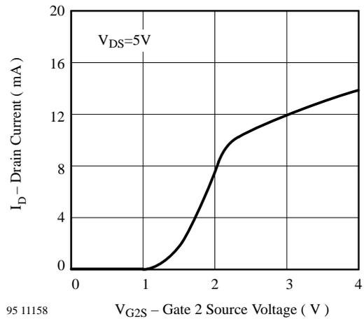
Figure 3. Drain Current vs. Gate 2 Source Voltage
