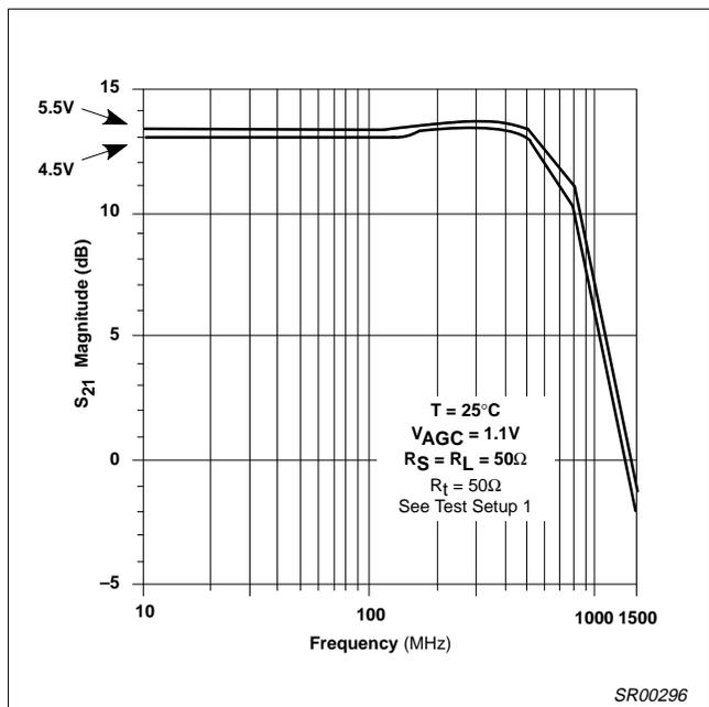
Figure 24. Insertion Gain vs Frequency and  $V_{CC}$
