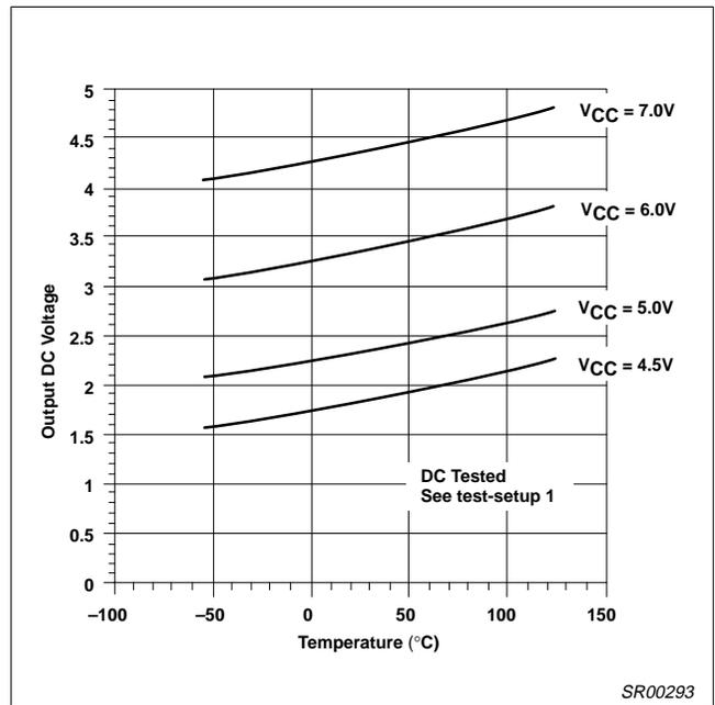
Figure 21. Output Bias Voltage vs Temperature and V<sub>CC</sub>
