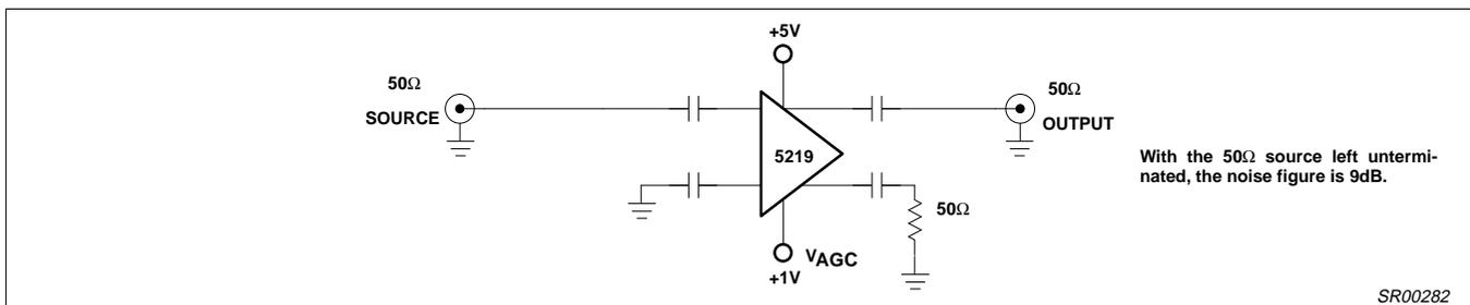
Figure 10. Underterminated Configuration
