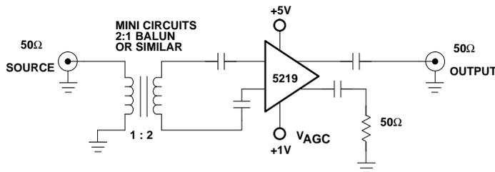
This circuit will exhibit about a 7dB noise figure with approximately 22dB gain.
