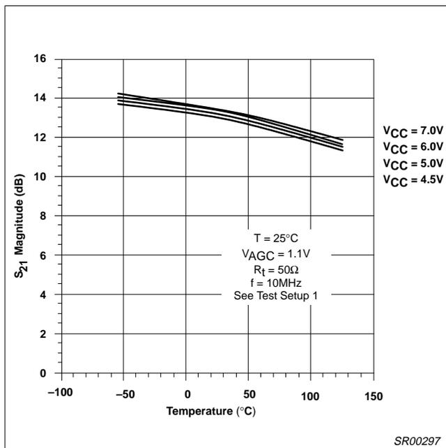
Figure 25. Insertion Gain vs Temperature and  $V_{CC}$
