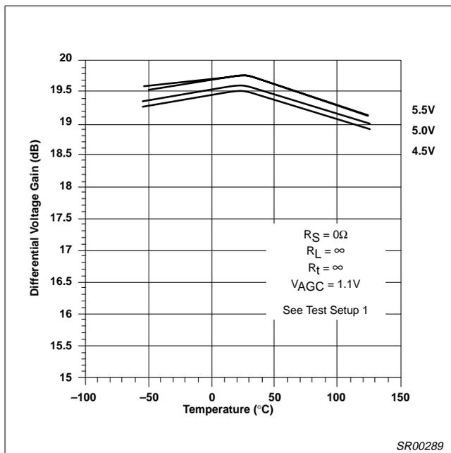
Figure 17. Voltage Gain vs Temperature and  $V_{CC}$
