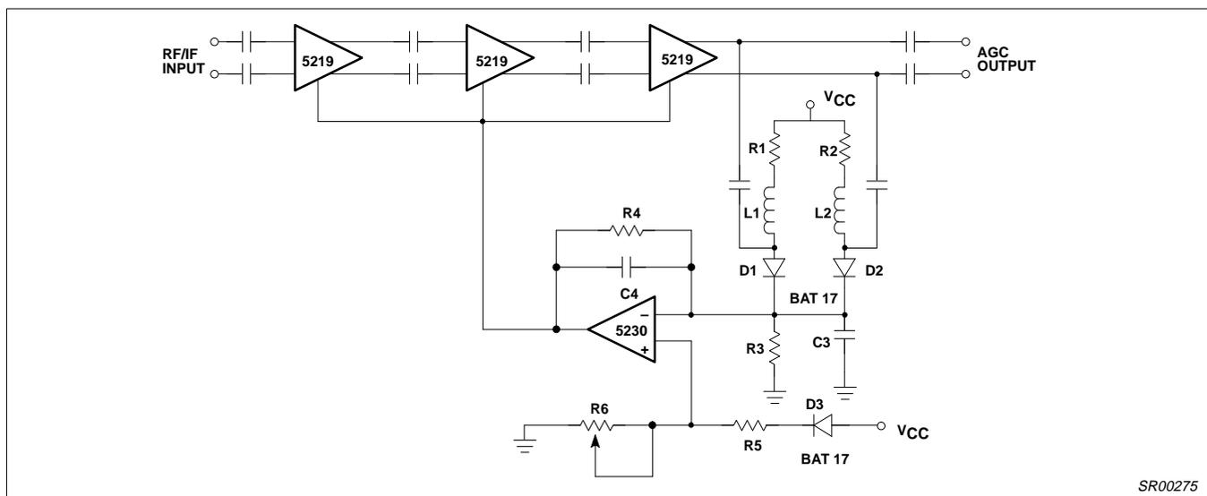
Figure 3. AGC Configuration Using Cascaded NE5219s
