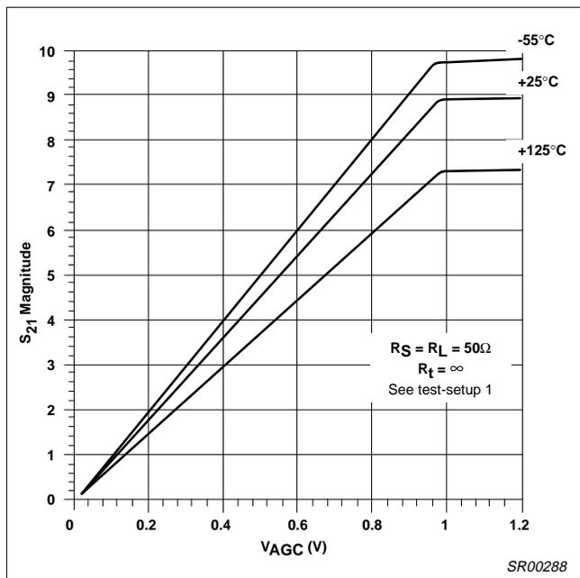
Figure 16. Insertion Gain vs  $V_{AGC}$  and Temperature
