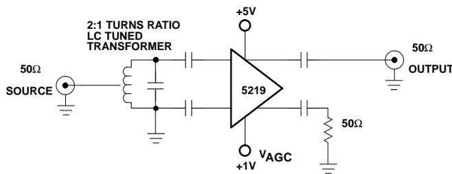
This circuit will exhibit about a 7dB noise figure with approximately 22dB gain. Narrowband circuits have the advantage of greater stability, particularly when multiple devices are cascaded.
