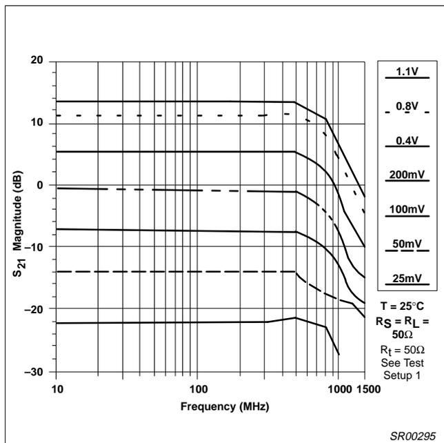
Figure 23. Insertion Gain vs Frequency and  $V_{AGC}$
