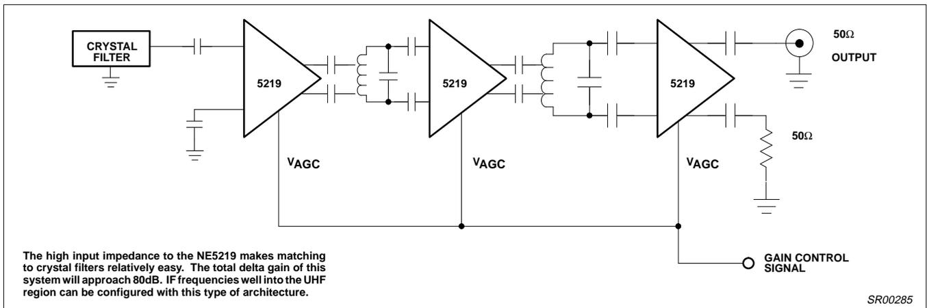
The high input impedance to the NE5219 makes matching to crystal filters relatively easy. The total delta gain of this system will approach 80dB. IF frequencies well into the UHF region can be configured with this type of architecture.
