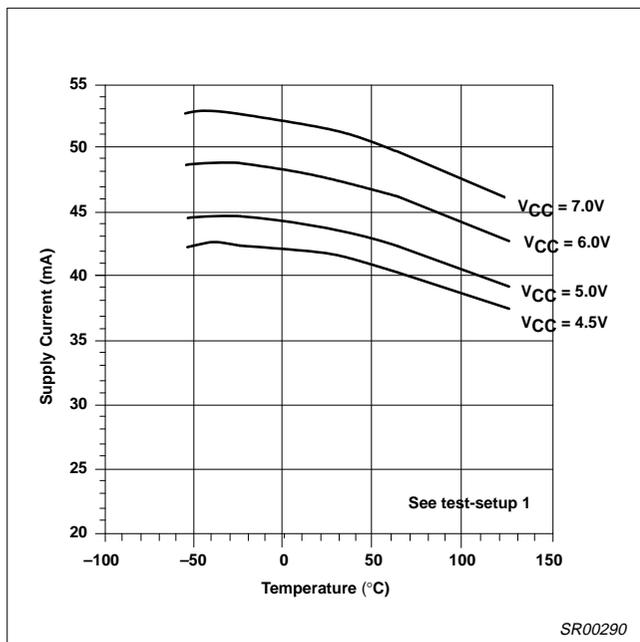
Figure 18. Supply Current vs Temperature and  $V_{CC}$
