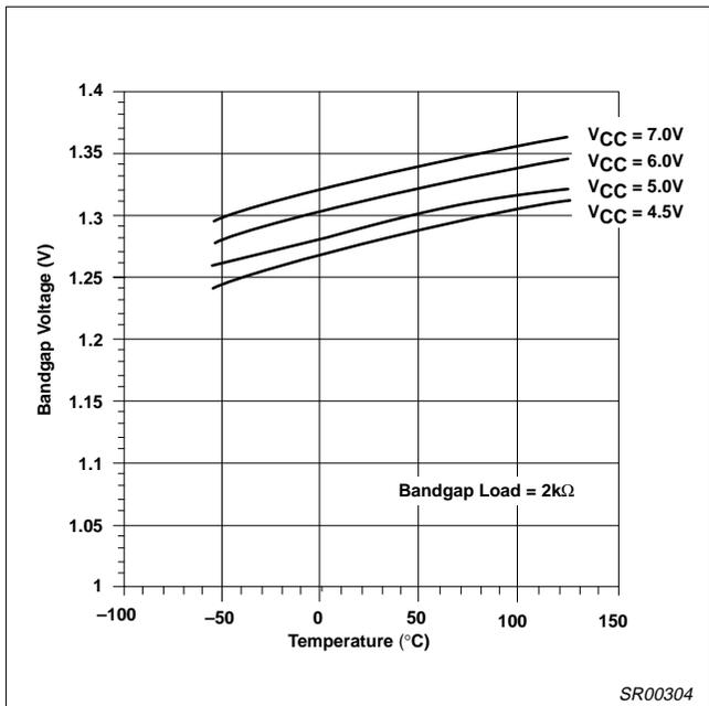
Figure 32. Bandgap Voltage vs Temperature and V<sub>CC</sub>
