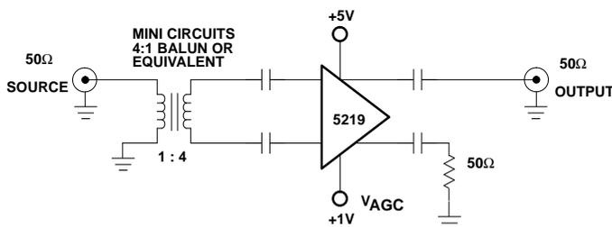
This circuit will exhibit about an 8dB noise figure with 24dB gain.
