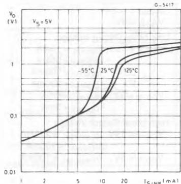
**Figure 5 :** Low Output Voltage Vs. Output Sink Current.
