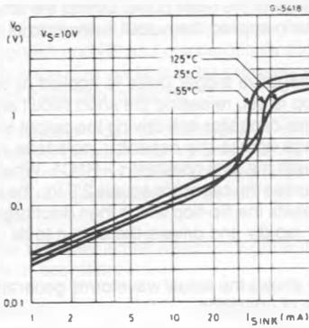
**Figure 6 :** Low Output Voltage Vs. Output Sink Current.
