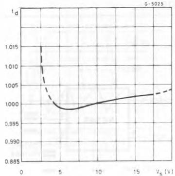
**Figure 9 :** Propagation Delay Vs. Voltage Level of Trigger Value.
