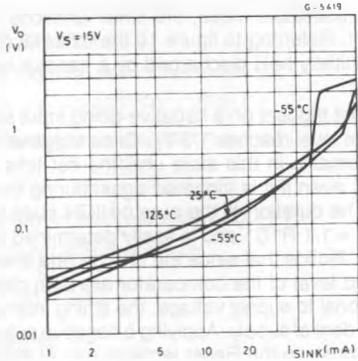
**Figure 7 :** High Output Voltage Drop Vs. Output Source Current.
