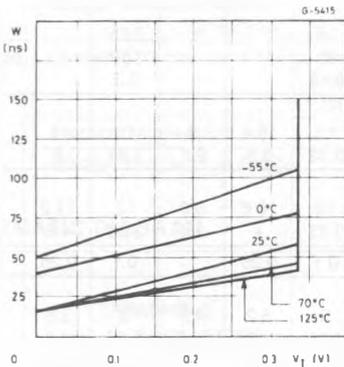
Figure 3 : Delay Time Vs. Temperature.
