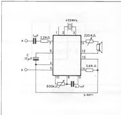
Figure 4 : Circuit Connection Scheme for Repetition Frequency Adjustment Described in Section 5.
