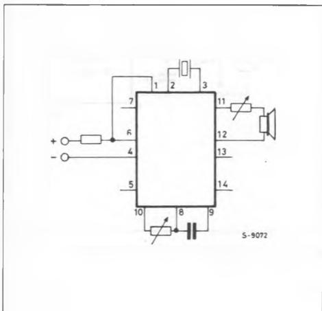
Figure 2 : SAA1094 with Power Supplied by the AC Ringing Signal..
