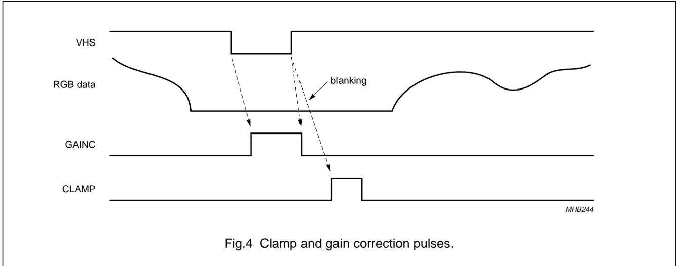
Fig.4 Clamp and gain correction pulses.
