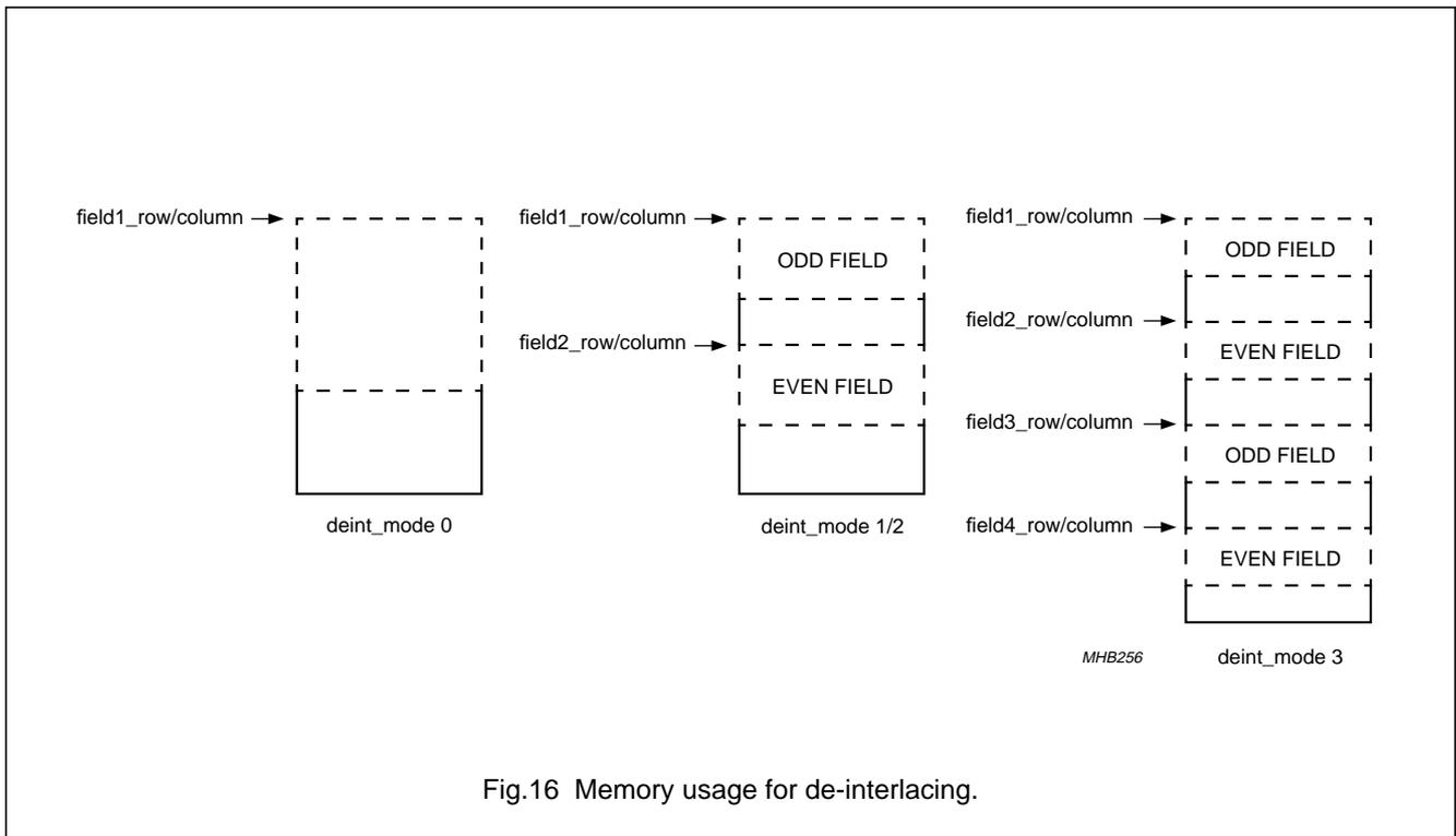
The memory interface addresses alternately the two banks of the SDRAM or SGRAM devices. So the memory needs for the field stores must be calculated from the following formula:
