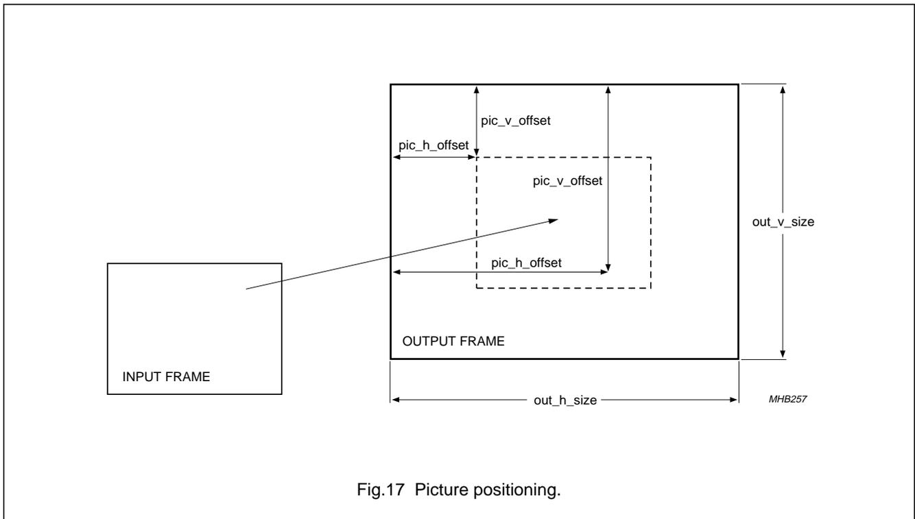
Fig.17 Picture positioning.
