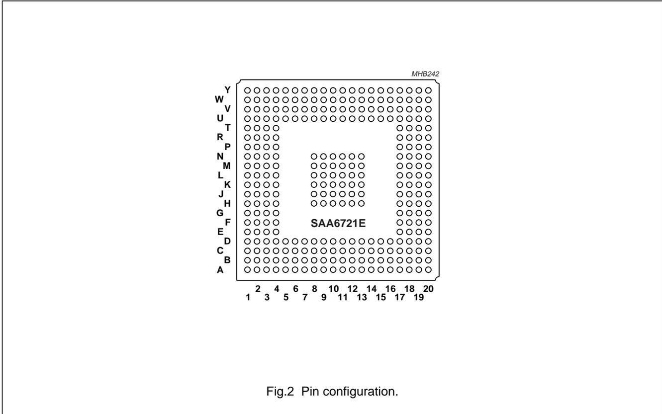
Fig.2 Pin configuration.
