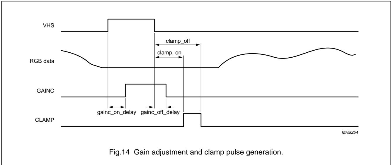
Fig.14 Gain adjustment and clamp pulse generation.
