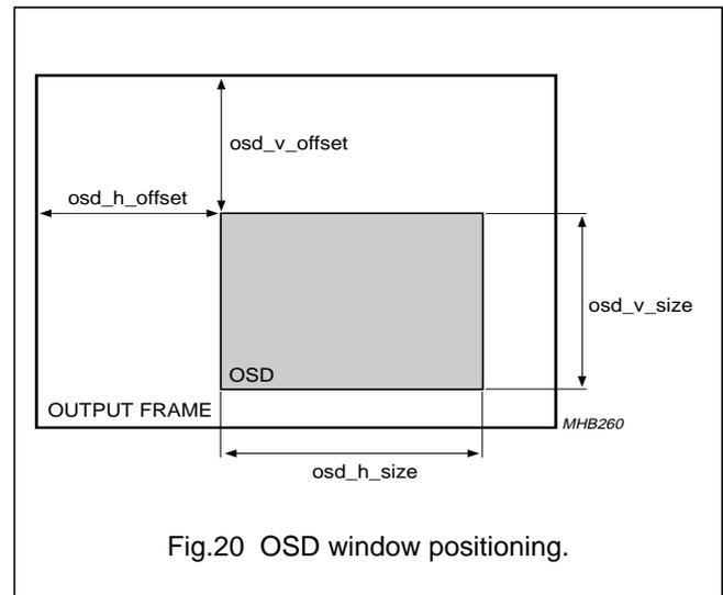
Fig.20 OSD window positioning.
