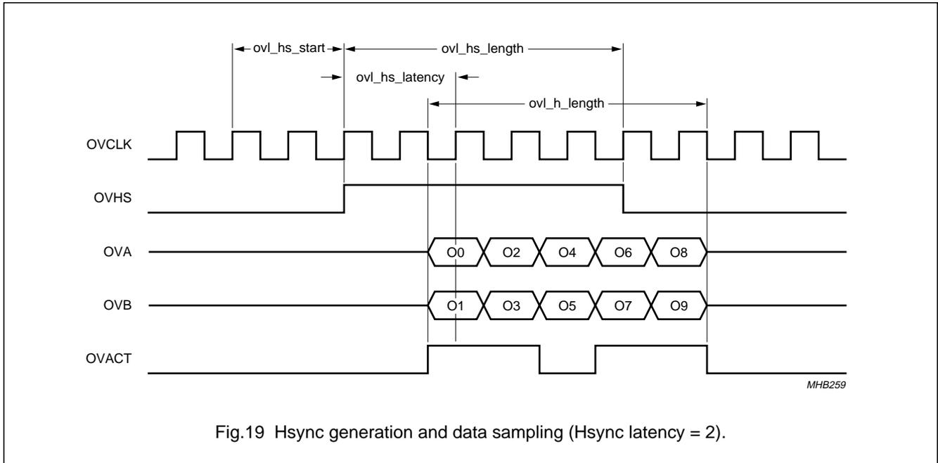
Fig.19 Hsync generation and data sampling (Hsync latency = 2).
