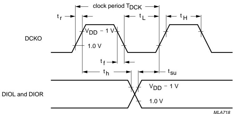
Fig.5 One bit code input timing.
