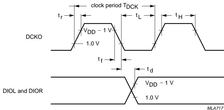
Fig.4 One bit code output timing.
