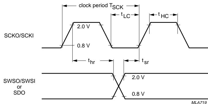
Fig.6 Serial output timing.
