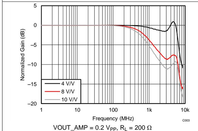
Figure 3. Differential Input Small-Signal Frequency Response vs Gain
