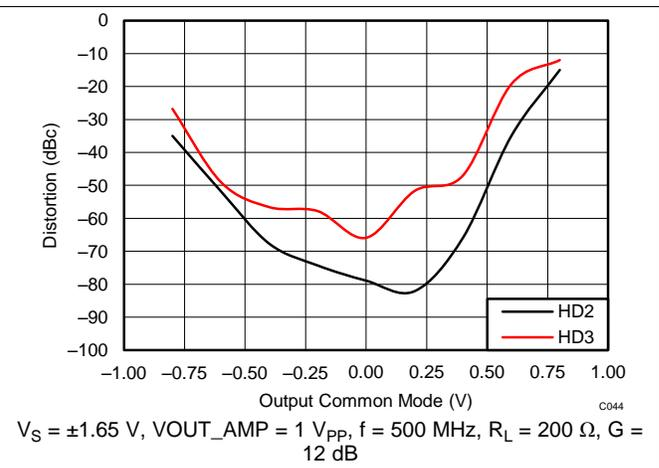
Figure 44. HD2 and HD3 vs Output Common-Mode Voltage
