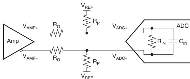
Figure 70. Resistor Network to DC Level-Shift Common-Mode Voltage
