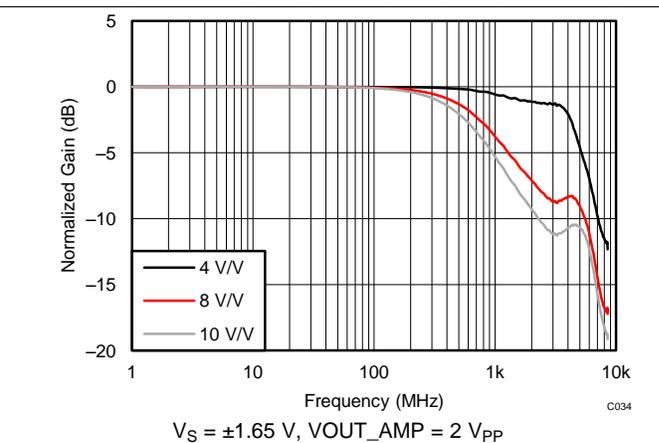
Figure 34. Large-Signal Differential Input Frequency Response vs  $R_L$
