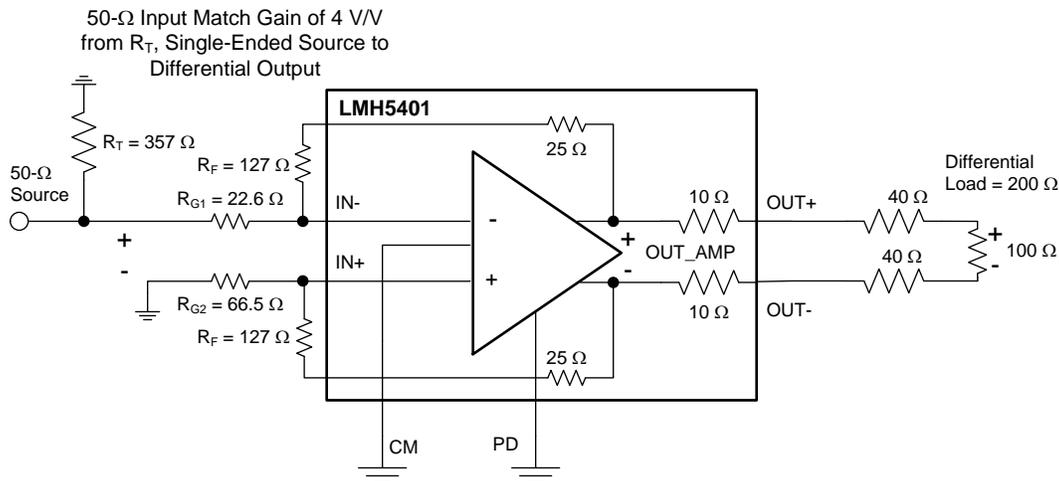
Figure 60. DC-Coupled, Single-Ended-to-Differential, Gain of 4 V/V
