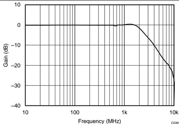
$V_S = \pm 1.65\text{ V}$ ,  $V_{OUT\_AMP} = 200\text{ mV}_{PP}$
