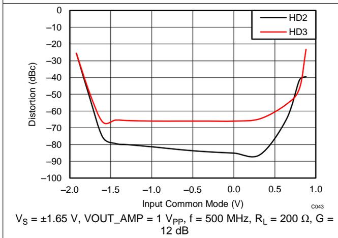
Figure 43. HD2 and HD3 vs Input Common-Mode Voltage
