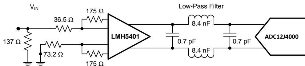
NOTE: Amplifier gain = 12 dB and net gain to ADC = 10.5 dB.
