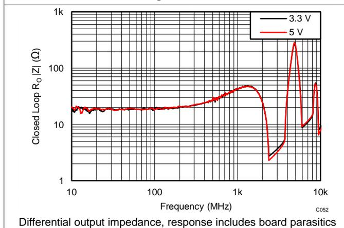
Figure 52. Differential Output Impedance vs Frequency
