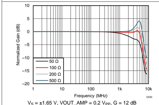
Figure 33. Small-Signal Differential Input Frequency Response vs  $R_L$
