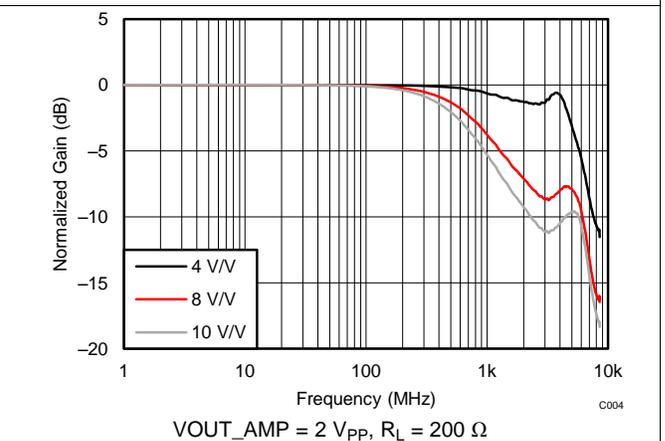
Figure 4. Differential Input Large-Signal Frequency Response vs Gain
