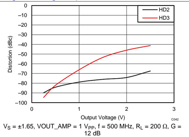
Figure 42. HD2 and HD3 vs Output Voltage
