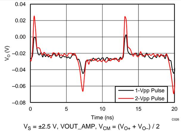
Figure 26. Pulse Response Common-Mode for Various  $V_O$
