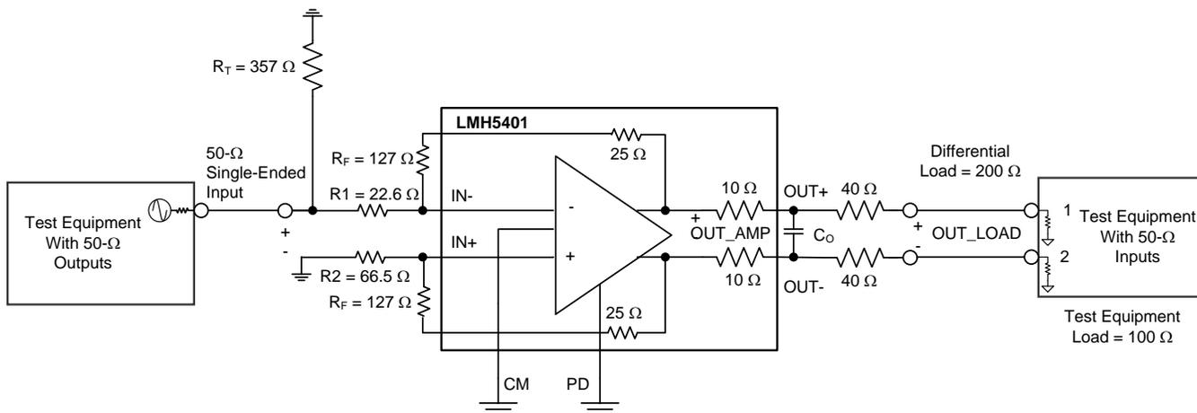
Figure 58. Test Schematic: Capacitive Load,  $A_V = 4 \text{ V/V}$
