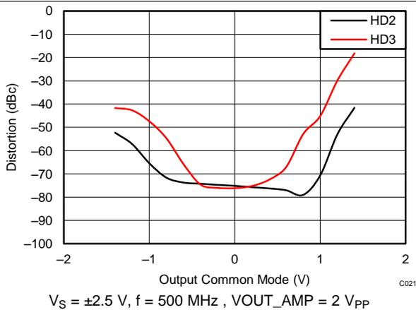
Figure 21. HD2 and HD3 vs Output Common-Mode Voltage
