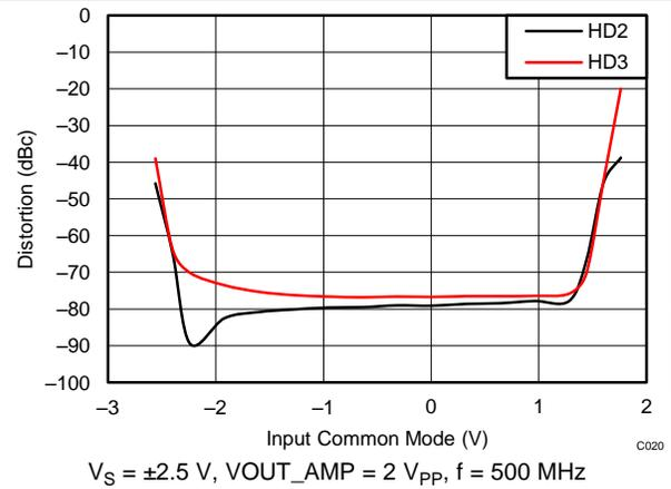
Figure 20. HD2 and HD3 vs Input Common-Mode Voltage
