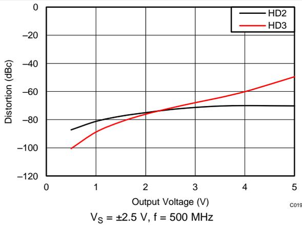
Figure 19. HD2 and HD3 vs Output Voltage
