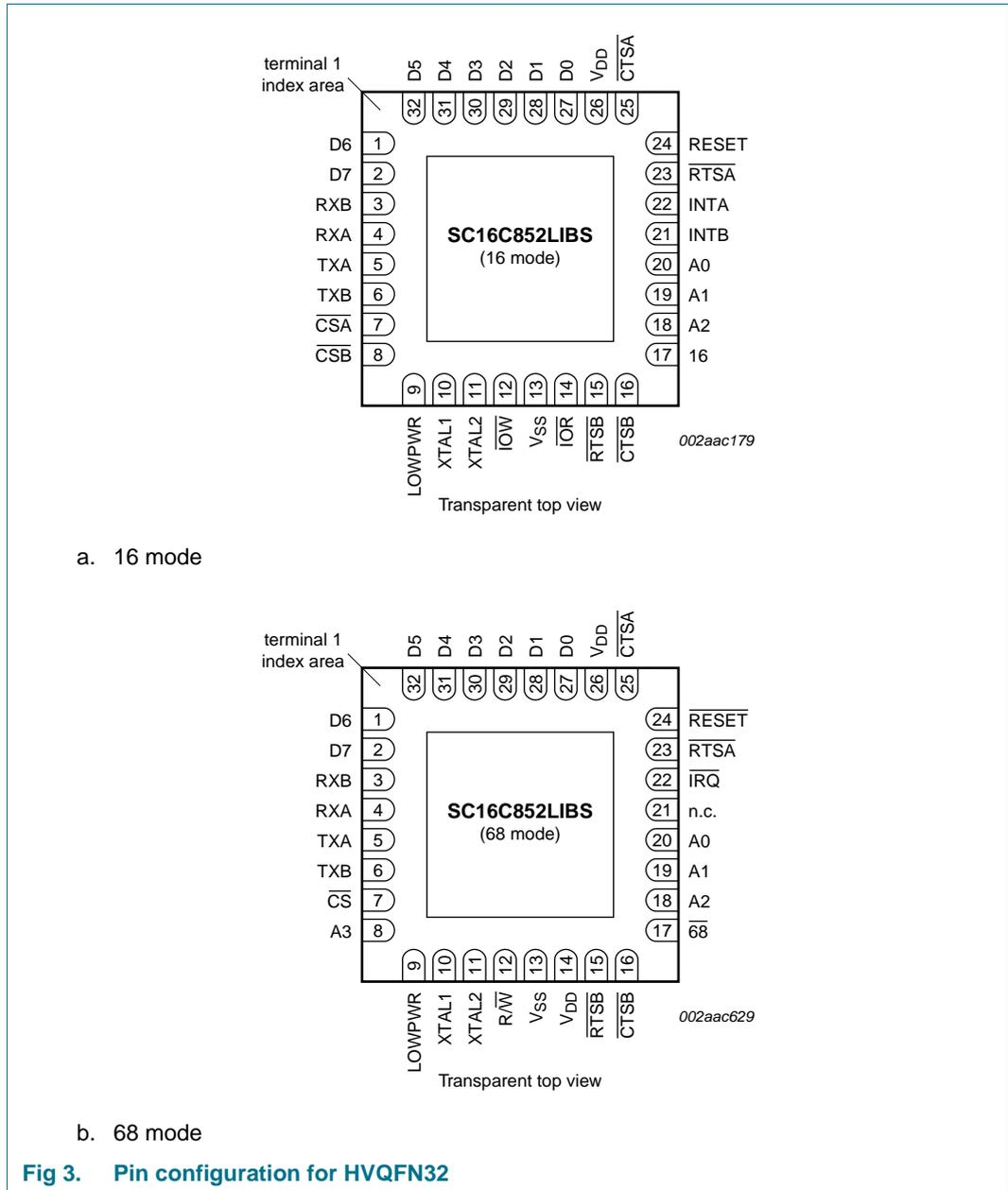
Fig 3. Pin configuration for HVQFN32
