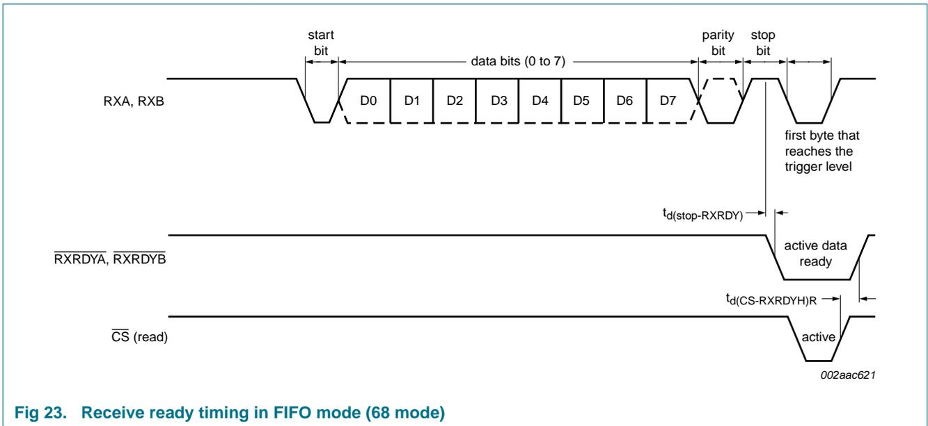
Fig 23. Receive ready timing in FIFO mode (68 mode)
