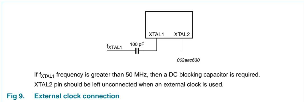
Fig 9. External clock connection
