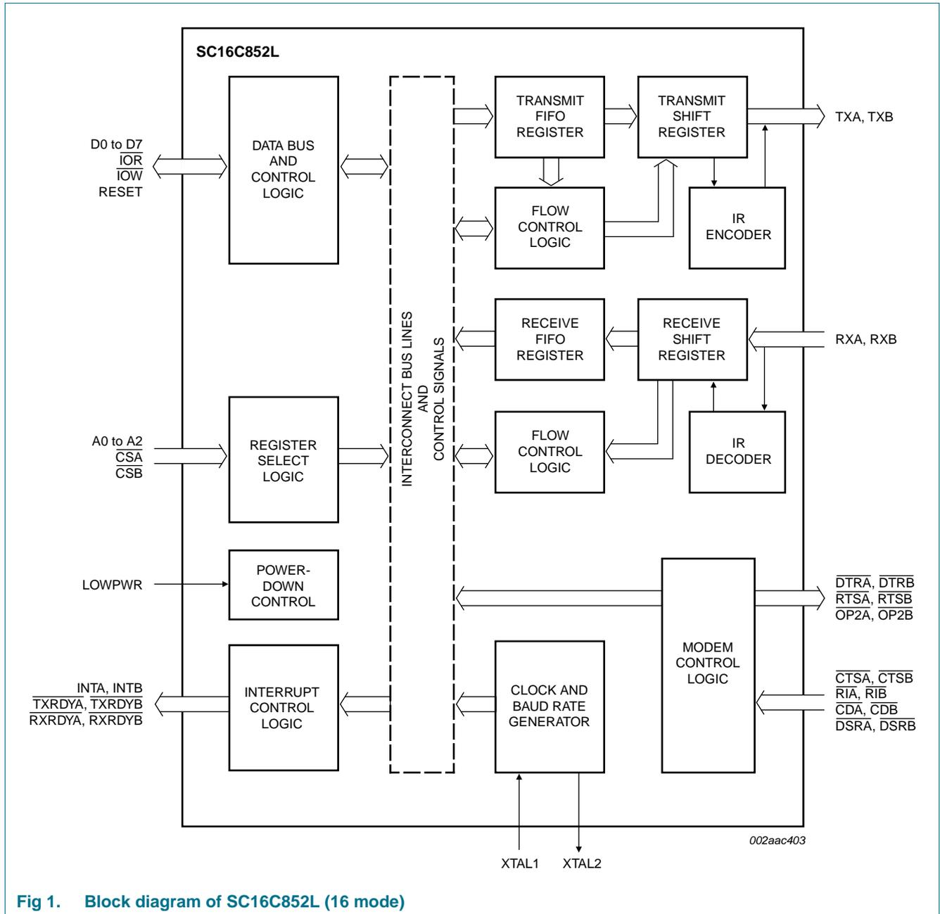
Fig 1. Block diagram of SC16C852L (16 mode)
