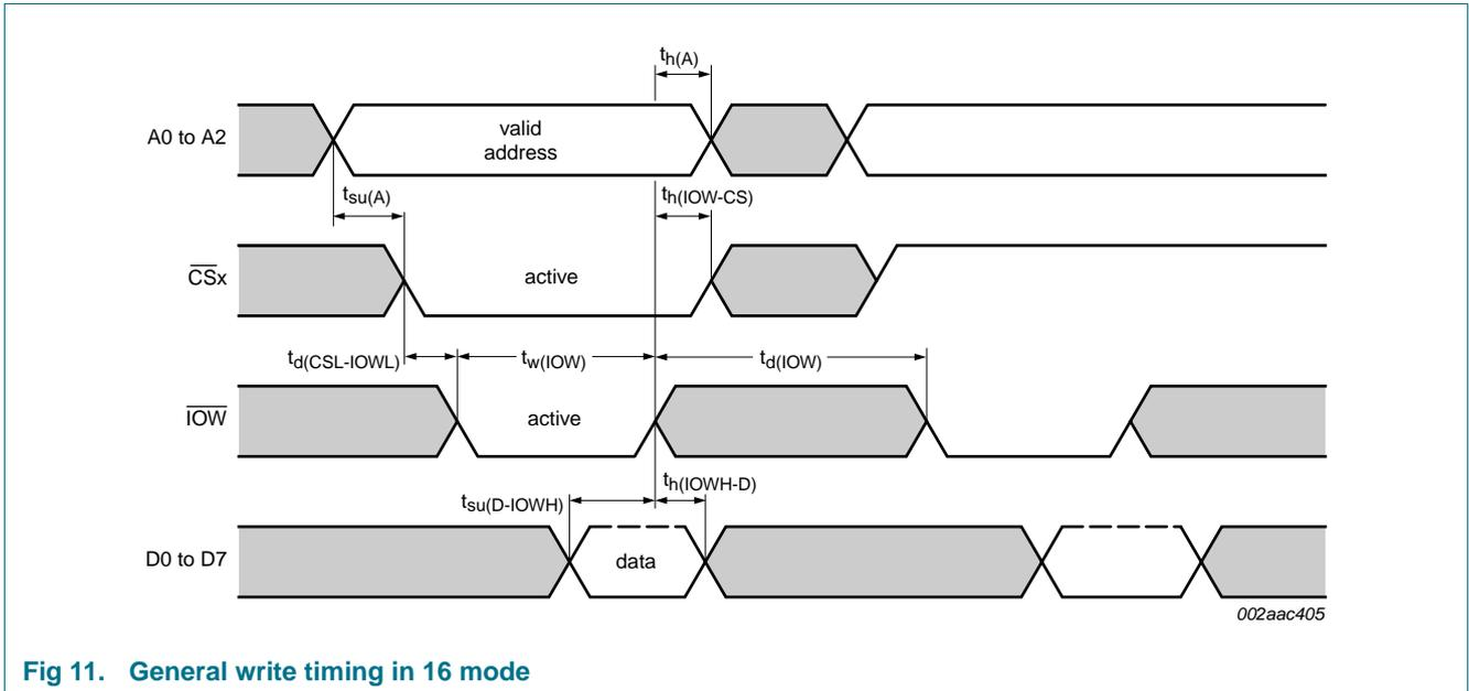
Fig 11. General write timing in 16 mode
