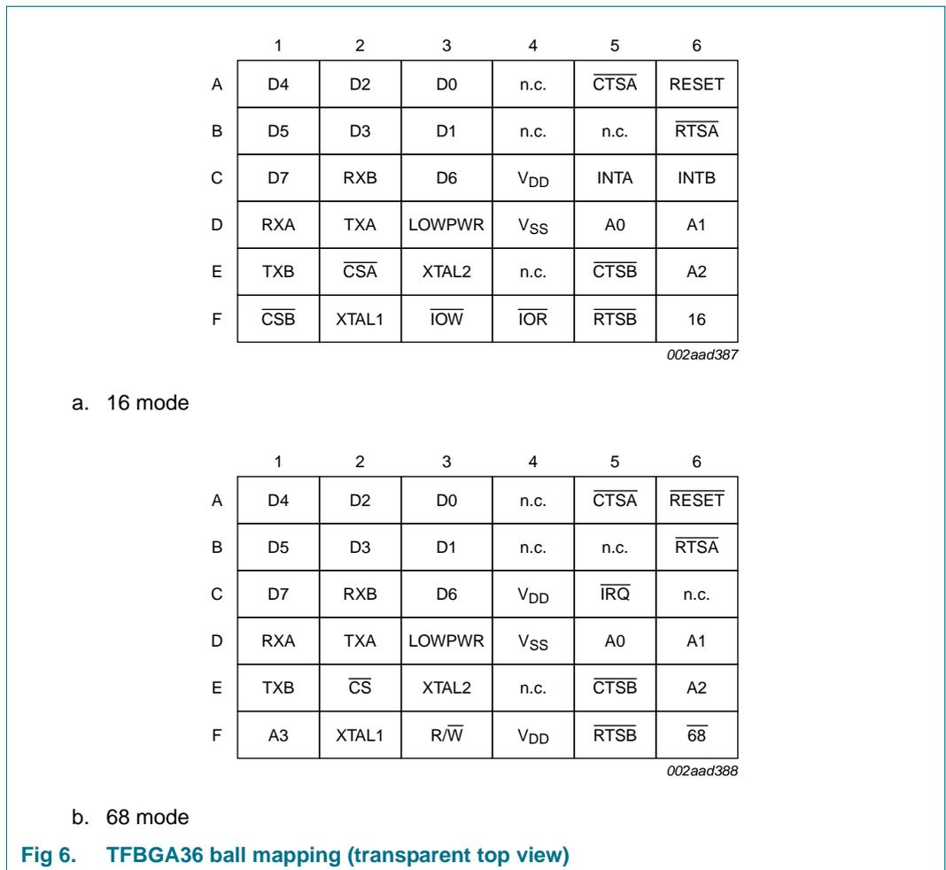
Fig 6. TFBGA36 ball mapping (transparent top view)
