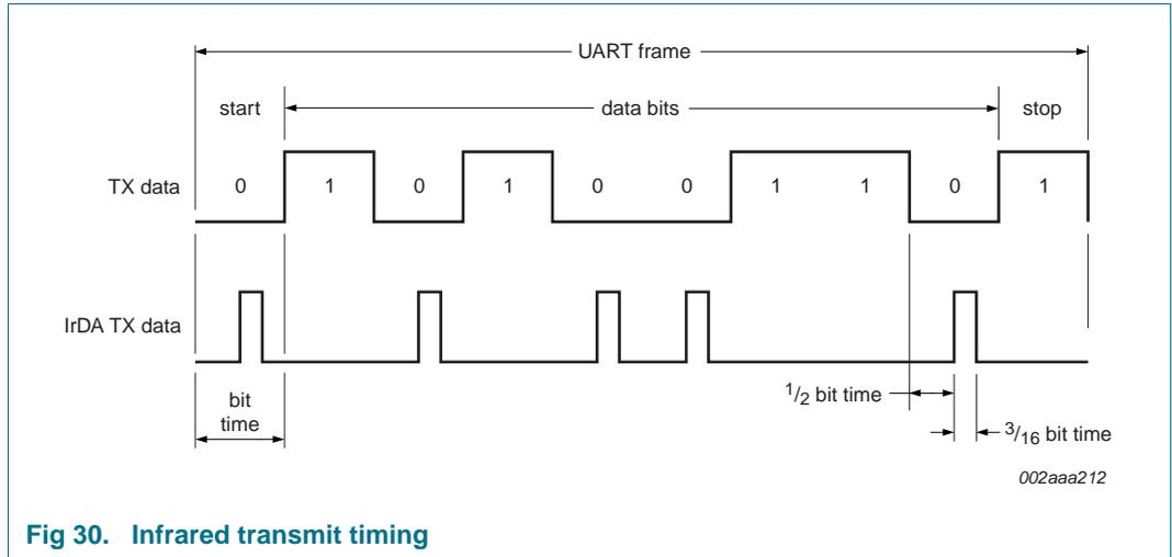
Fig 30. Infrared transmit timing
