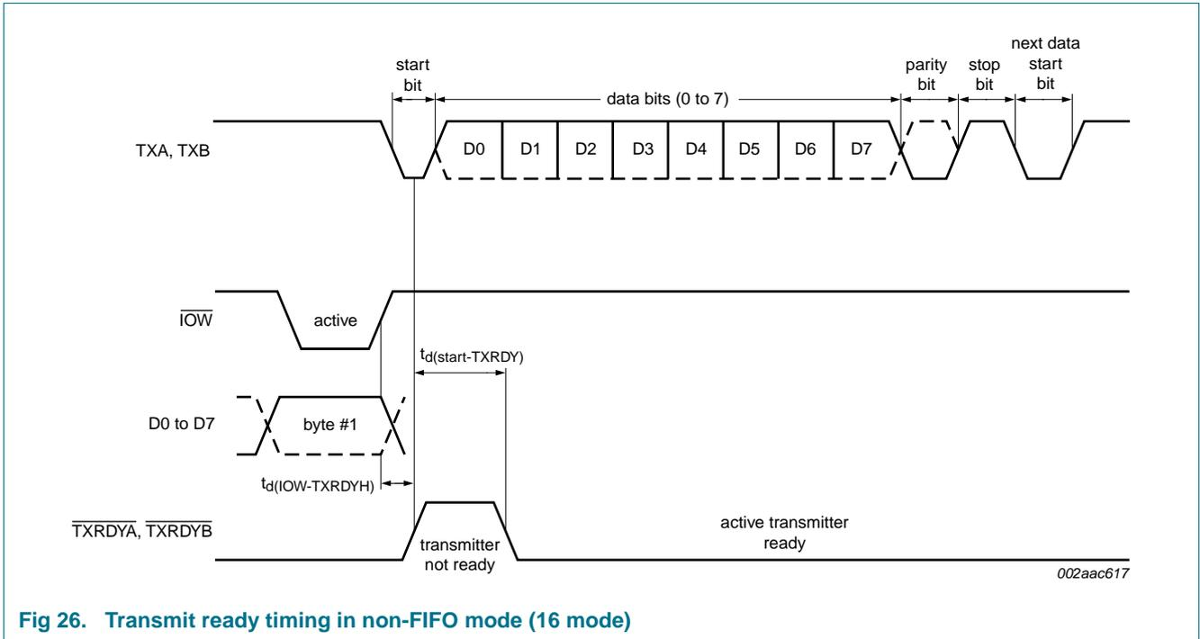
Fig 26. Transmit ready timing in non-FIFO mode (16 mode)
