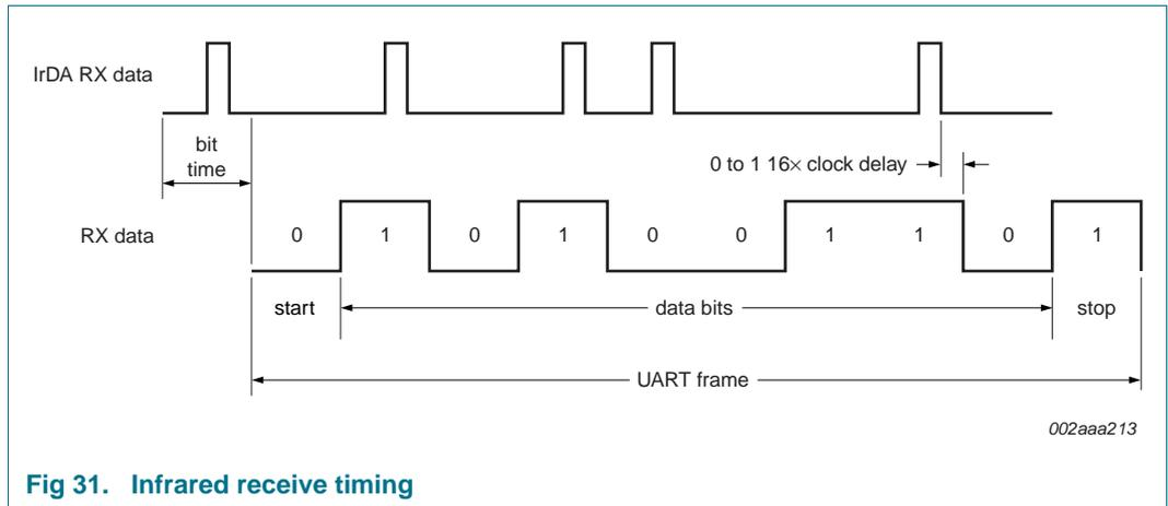
Fig 31. Infrared receive timing
