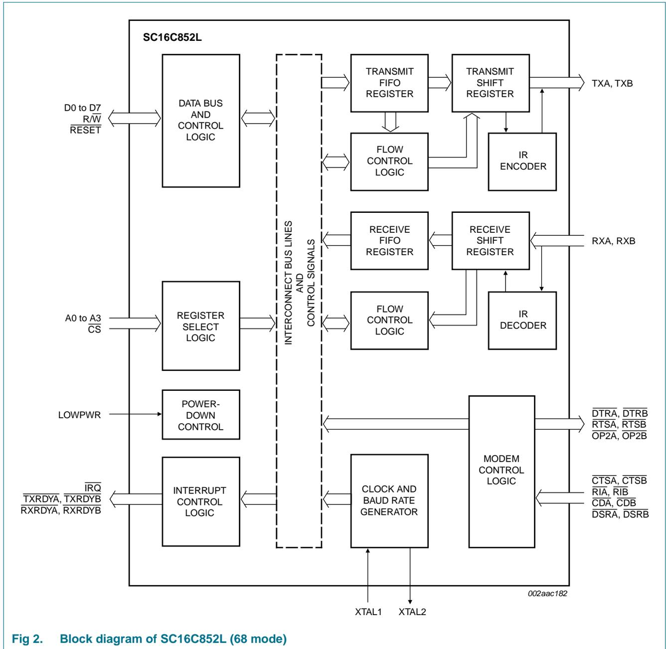
Fig 2. Block diagram of SC16C852L (68 mode)
