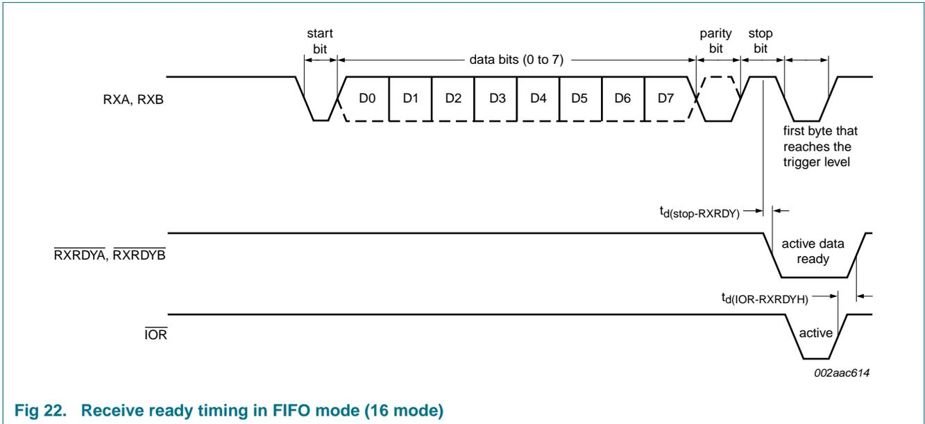
Fig 22. Receive ready timing in FIFO mode (16 mode)
