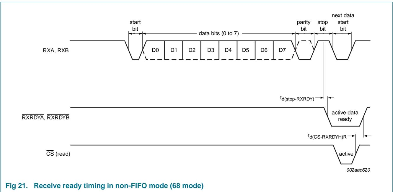
Fig 21. Receive ready timing in non-FIFO mode (68 mode)
