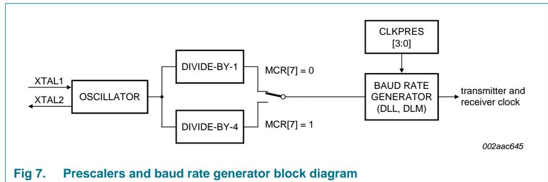
Fig 7. Prescalers and baud rate generator block diagram
