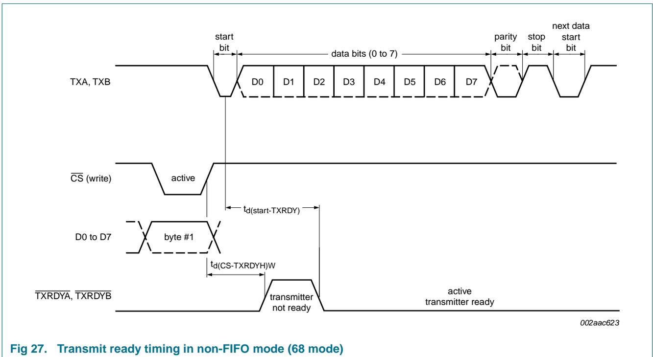
Fig 27. Transmit ready timing in non-FIFO mode (68 mode)
