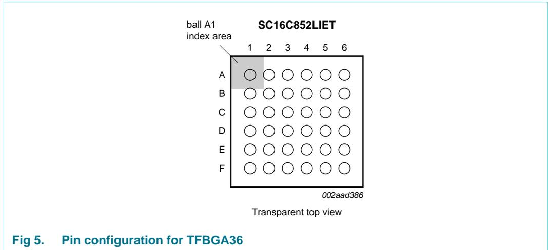
Fig 5. Pin configuration for TFBGA36
