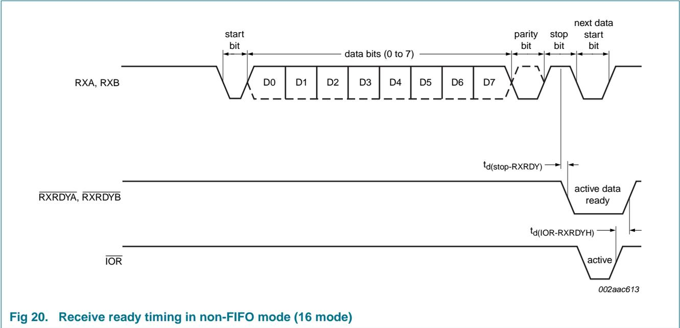
Fig 20. Receive ready timing in non-FIFO mode (16 mode)
