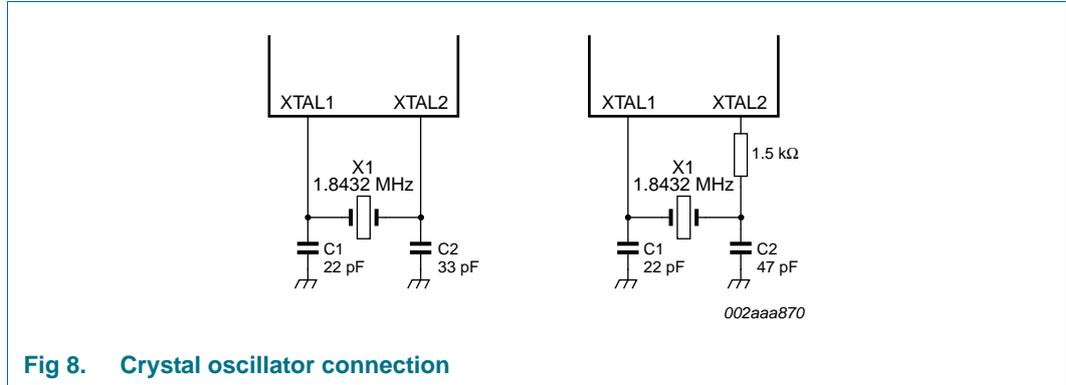
Fig 8. Crystal oscillator connection
