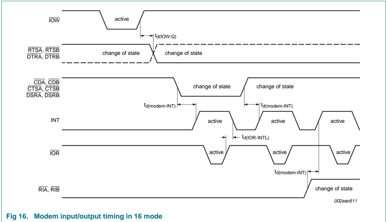
Fig 16. Modem input/output timing in 16 mode
