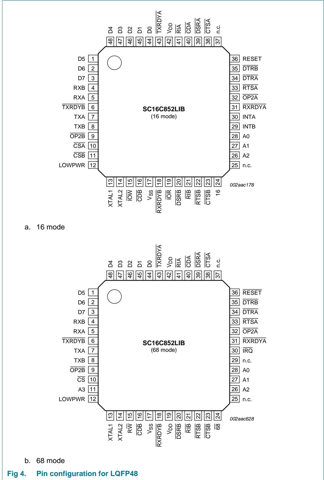
Fig 4. Pin configuration for LQFP48
