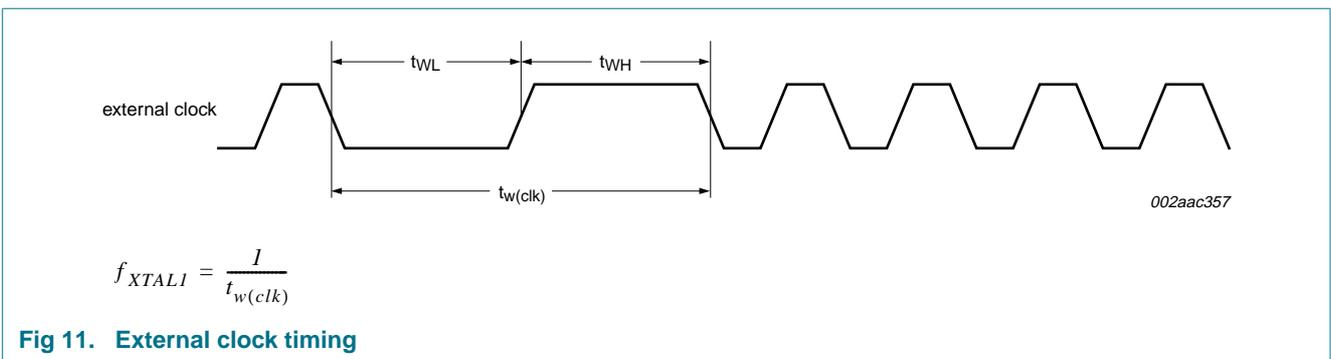
Fig 11. External clock timing
