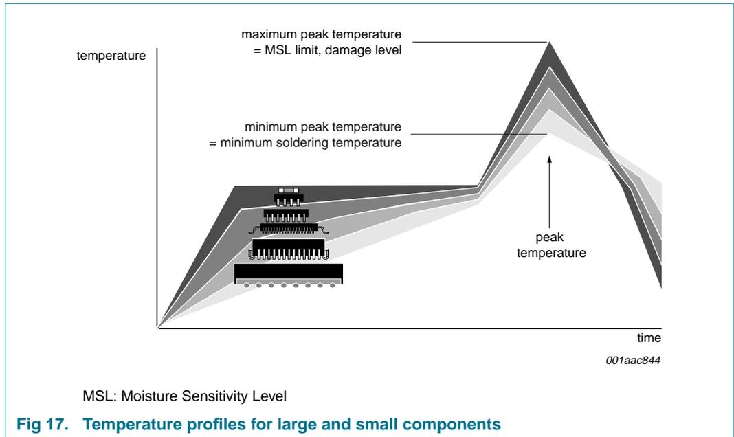
Fig 17. Temperature profiles for large and small components
