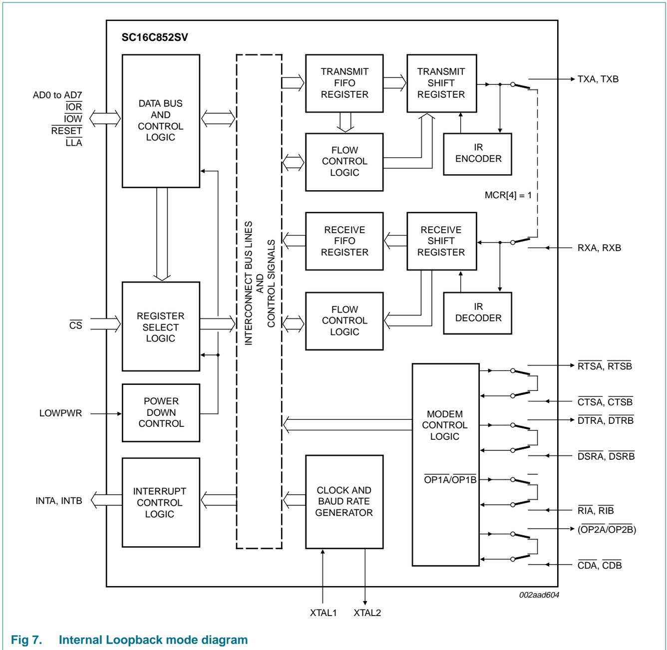
Fig 7. Internal Loopback mode diagram
