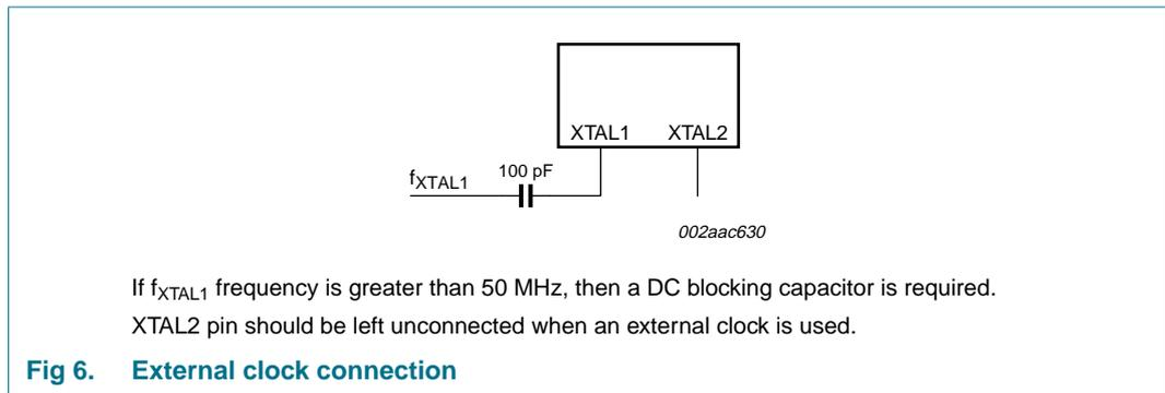
Fig 6. External clock connection
