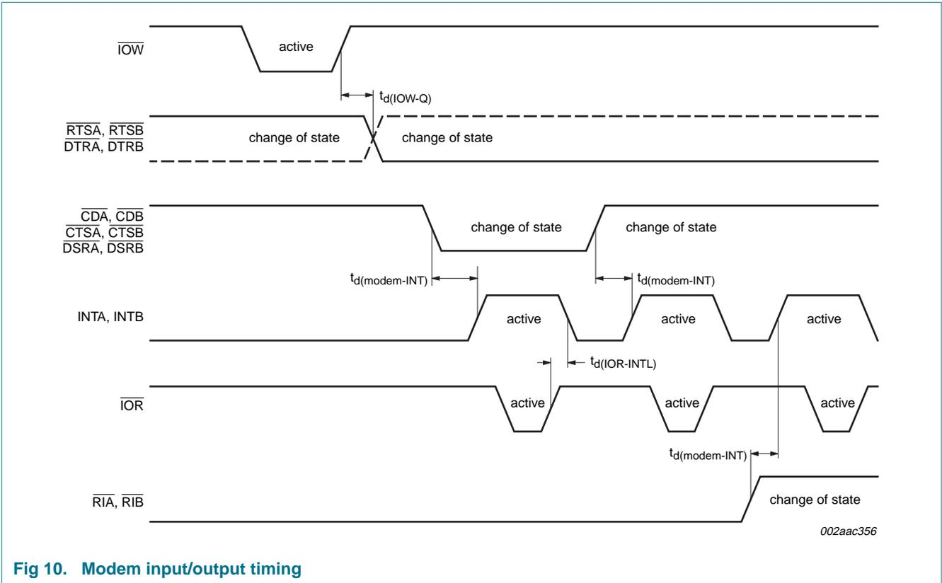
Fig 10. Modem input/output timing
