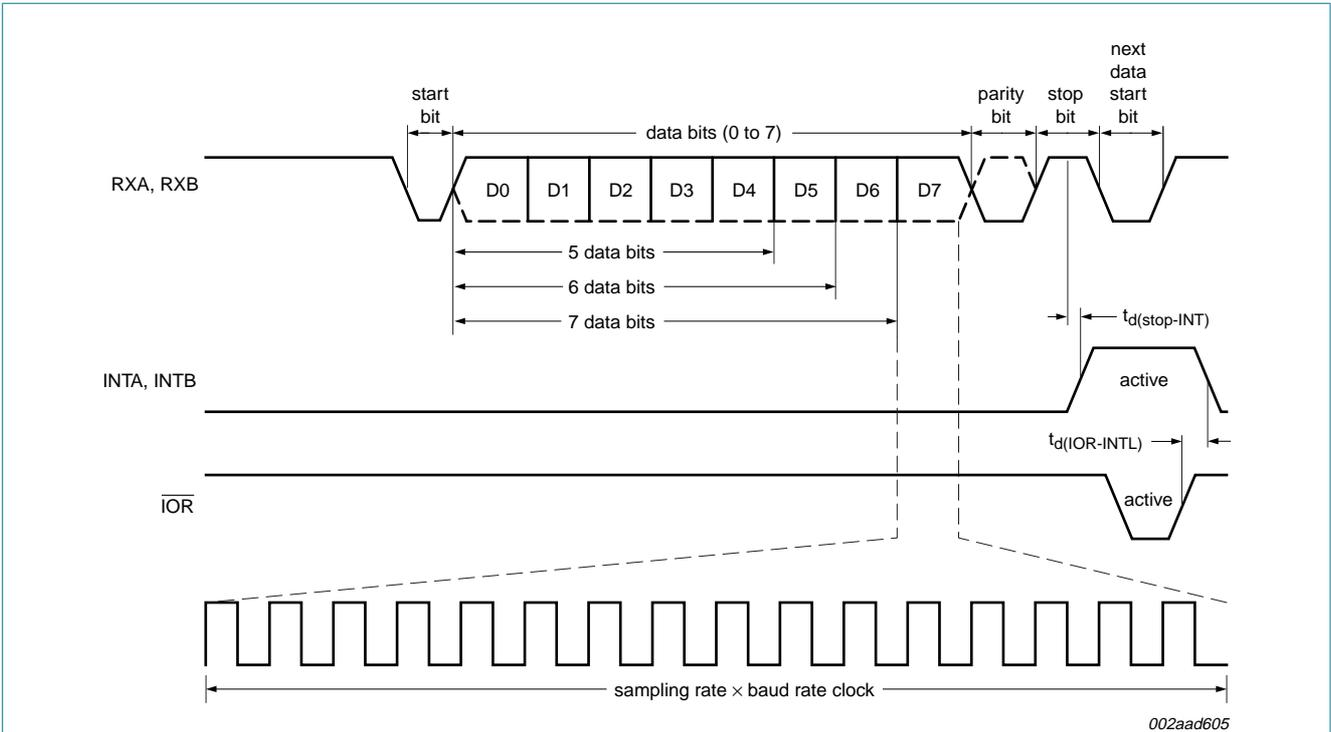
Fig 12. Receive timing
