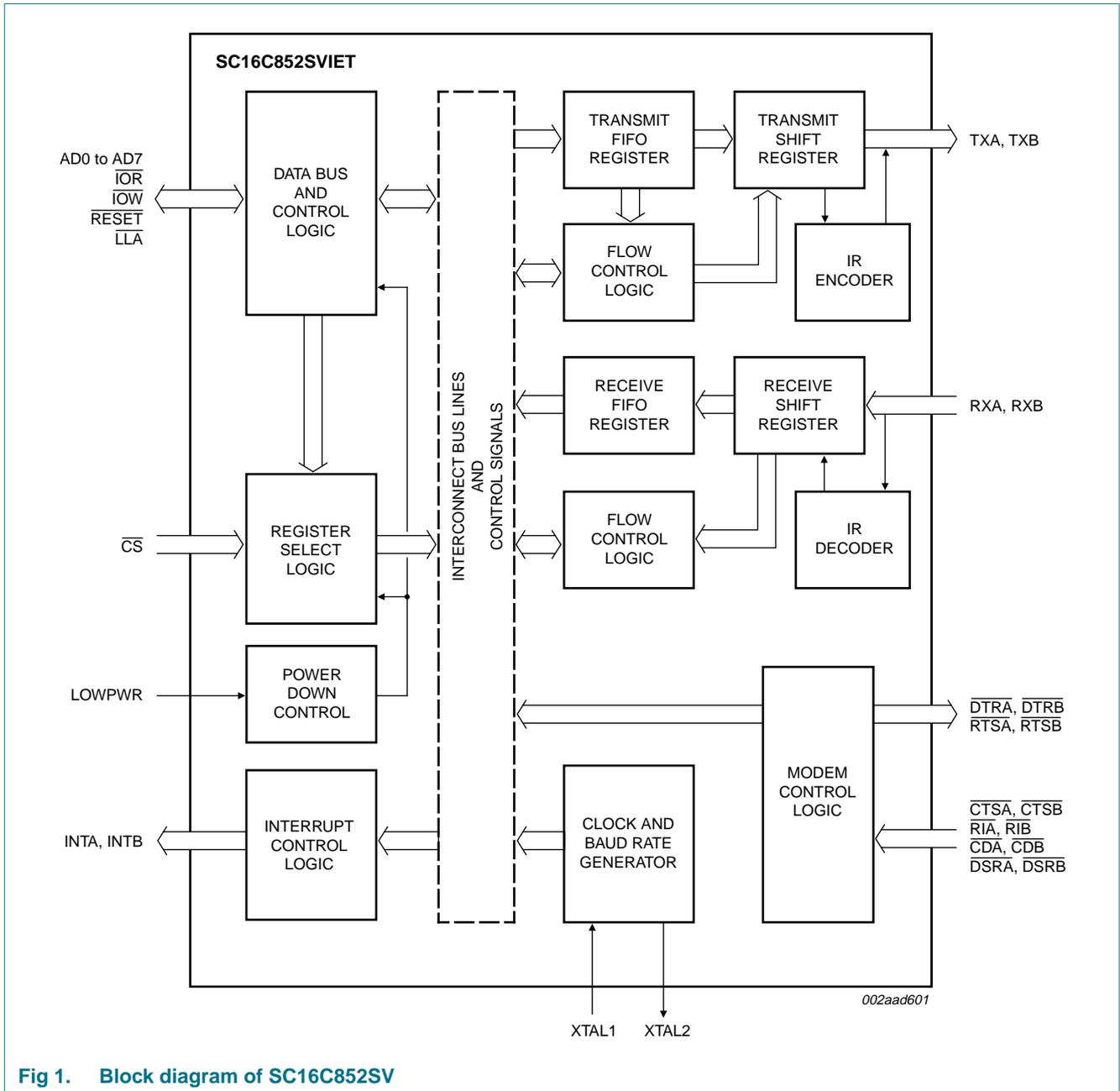
Fig 1. Block diagram of SC16C852SV
