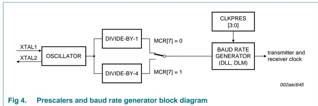
**Fig 4. Prescalers and baud rate generator block diagram**
