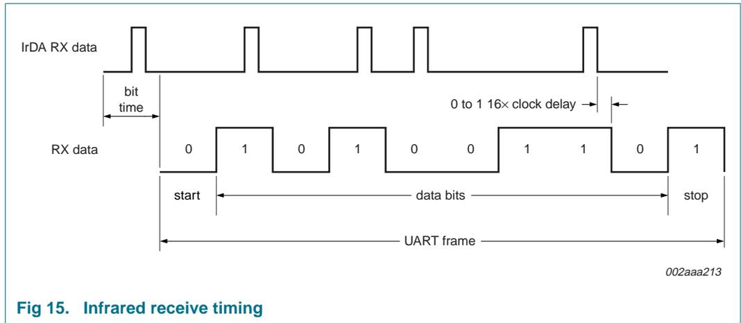
Fig 15. Infrared receive timing
