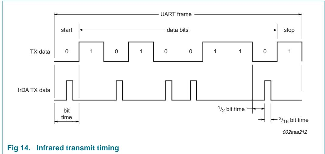
Fig 14. Infrared transmit timing
