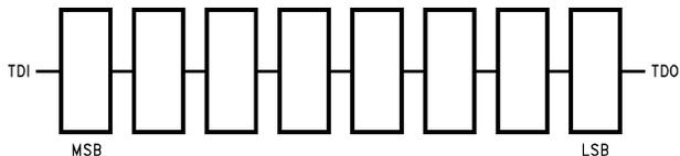
Figure 5. Instruction Register Scan Chain Definition
