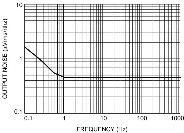
Figure 8. Output Voltage Noise 0.1 Hz - 1 kHz
