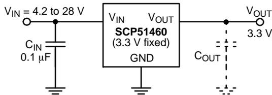
Table 6 shows the maximum capacitance of C<sub>OUT</sub> for various load currents to avoid instability.
