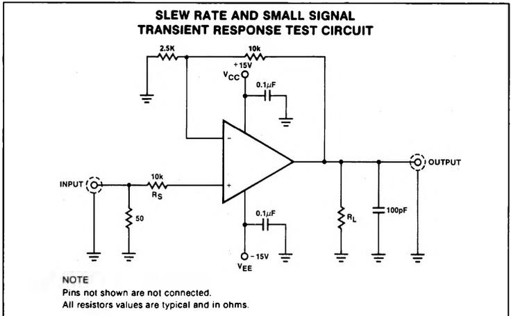
**TEST LOAD CIRCUITS (Cont'd)**
