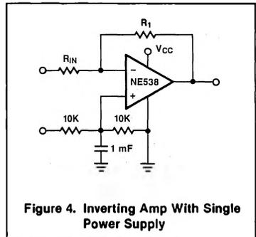
**Figure 4. Inverting Amp With Single Power Supply**
