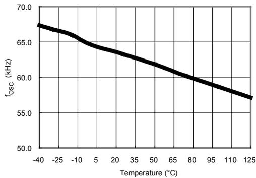
**Figure 11. Center Frequency (f<sub>OSC</sub>) vs. Temperature**
