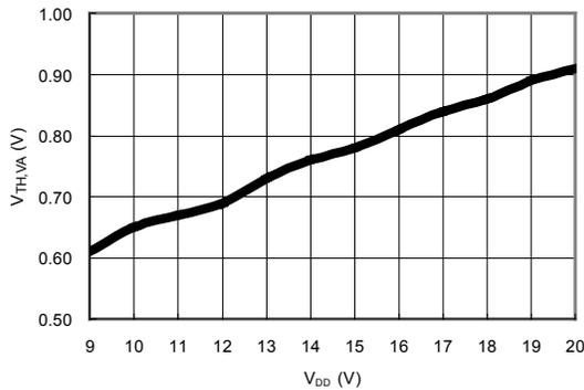
**Figure 17. Valley Threshold Voltage (V<sub>STHVA</sub>) vs. V<sub>DD</sub>**
