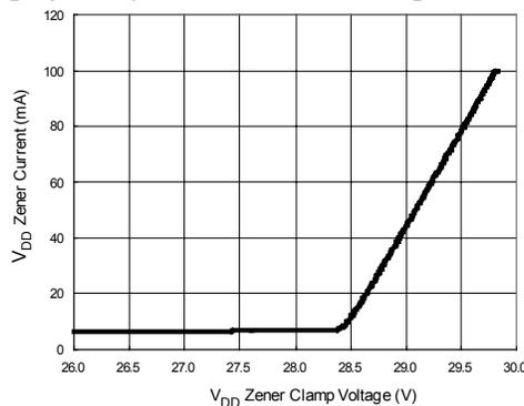
**Figure 19. V<sub>DD</sub> Zener Current vs. Zener Clamp Voltage**
