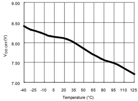
**Figure 8. Turn-off Threshold Voltage (V<sub>DD-OFF</sub>) vs. Temperature**
