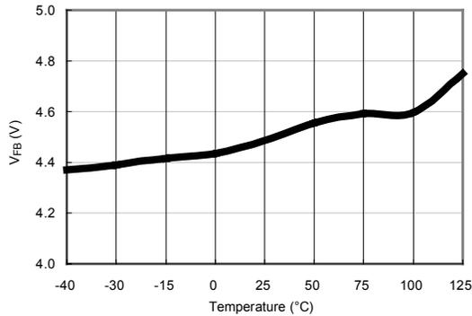
**Figure 13. FB Open-Loop Voltage (V<sub>FB</sub>) vs. Temperature**
