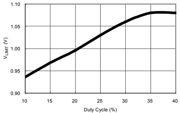
**Figure 18. V<sub>LIMIT</sub> Ramp vs. Duty Cycle**
