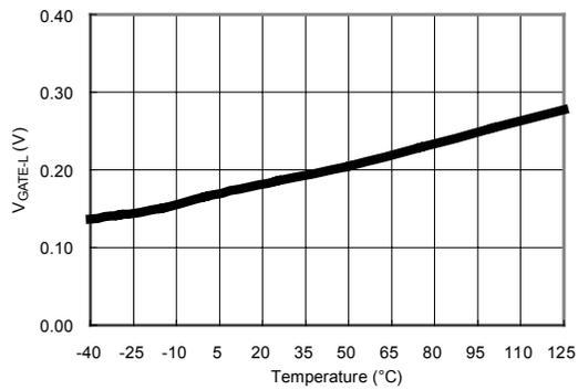
**Figure 15. Output Voltage Low (V<sub>GATE-L</sub>) vs. Temperature**
