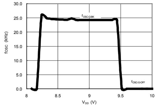
**Figure 16. Green-Mode Burst Back and Green-Mode Off Frequency vs. V<sub>DD</sub>**
