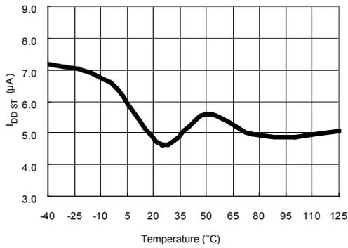
**Figure 9. Startup Current (I<sub>DD-ST</sub>) vs. Temperature**
