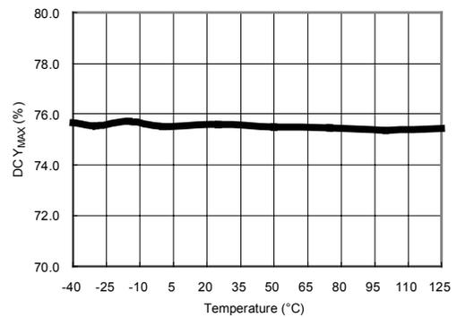
**Figure 12. Maximum Duty Cycle (DCY<sub>MAX</sub>) vs. Temperature**
