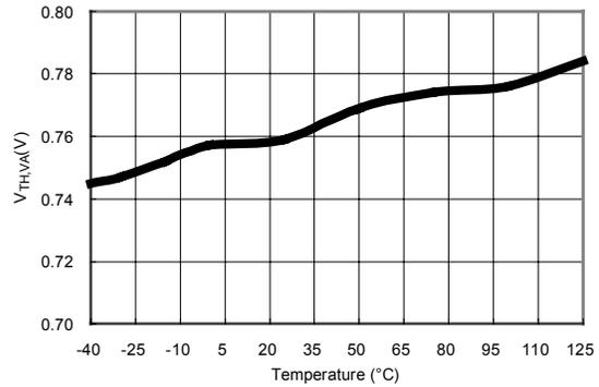
**Figure 14. Valley Threshold Voltage (V<sub>STHVA</sub>) vs. Temperature**
