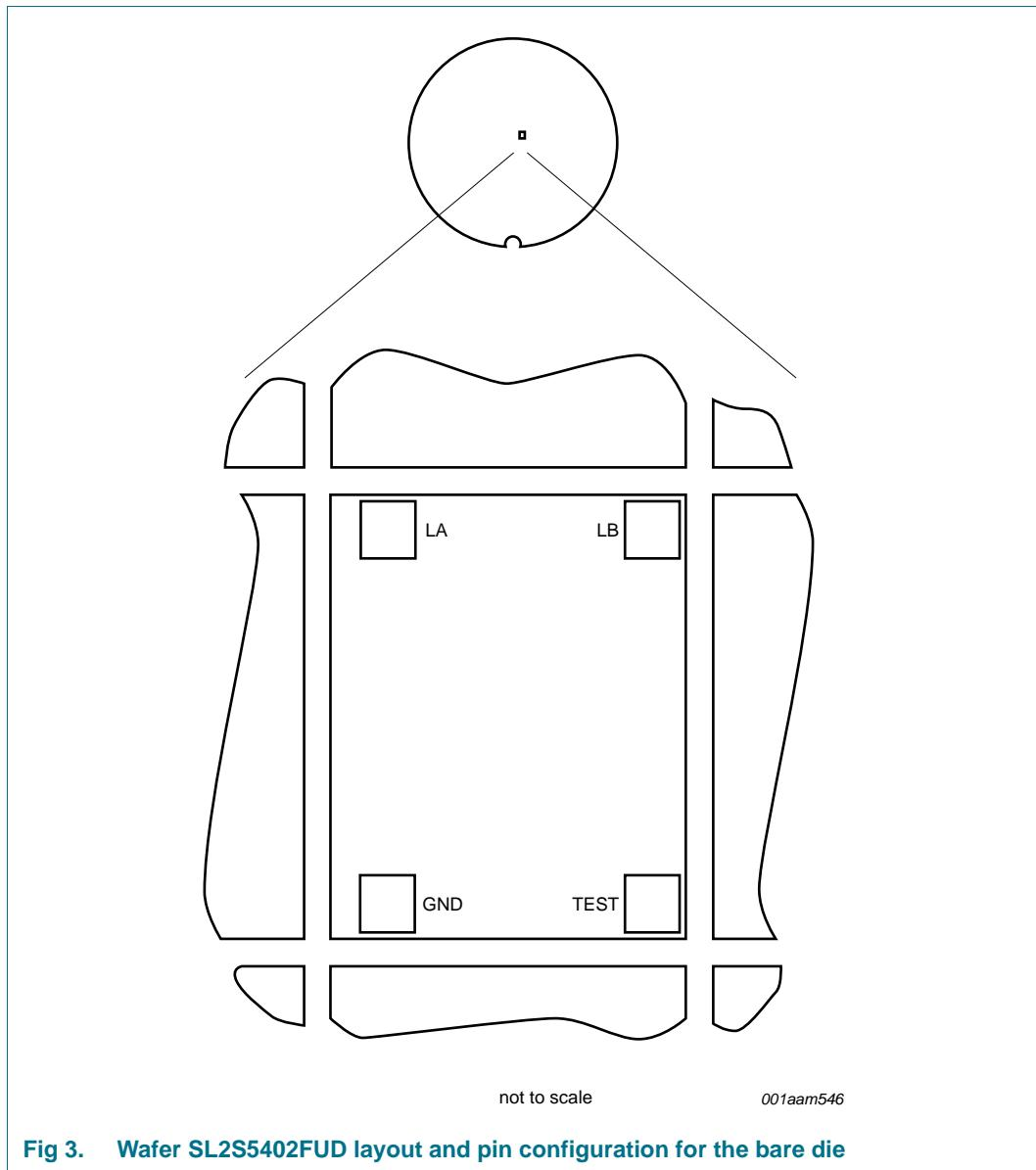
Fig 3. Wafer SL2S5402FUD layout and pin configuration for the bare die
