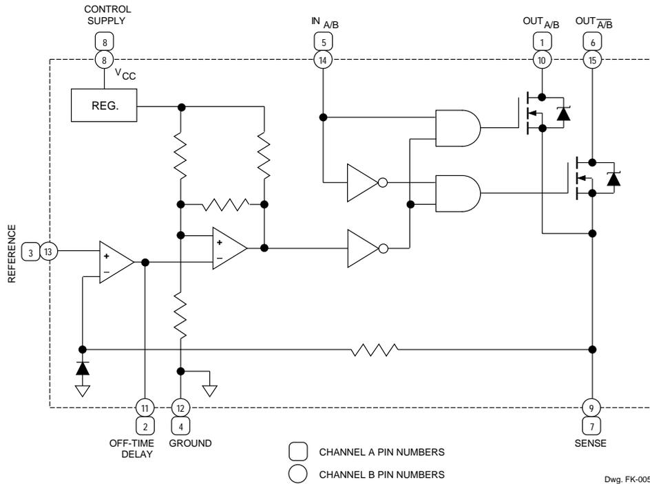
Note that except for the control supply, channels A and B are electrically isolated.
