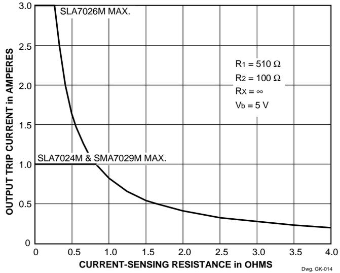
**FIGURE 3. CURRENT-SENSING RESISTANCE**
