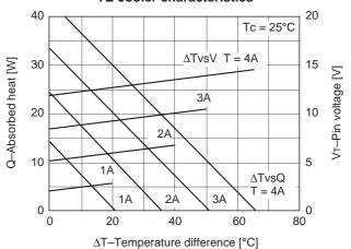
Tth: Thermistor temperature Tc : Case temperature
