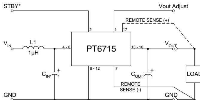
$C_{in}$  = Required 1000 $\mu$ F electrolytic
