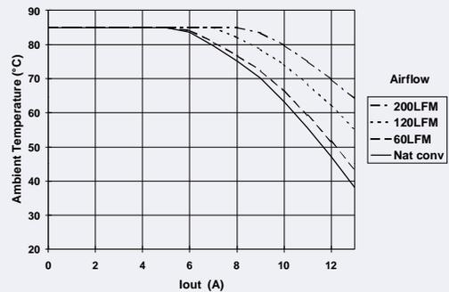
Note A: Characteristic data has been developed from actual products tested at 25°C. This data is considered typical data for the Converter.
