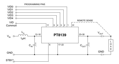
$C_{in}$  = Required 1500 $\mu$ F electrolytic
