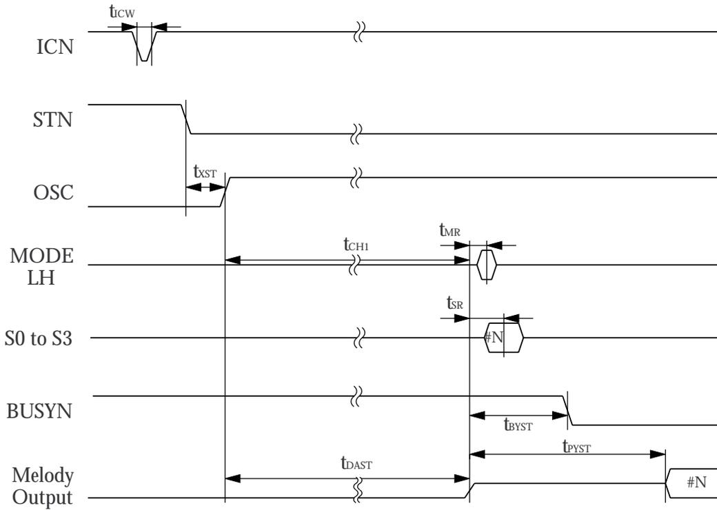
Figure 21. Level hold mode (standby to melody start)
