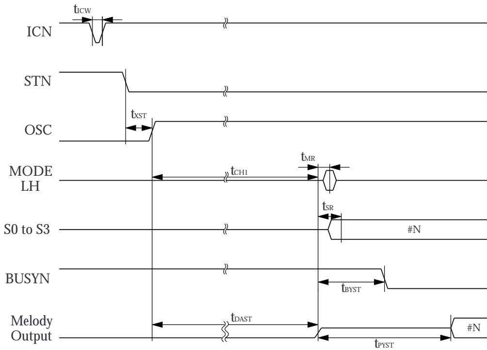
Figure 19. Level hold mode (standby to melody start)
