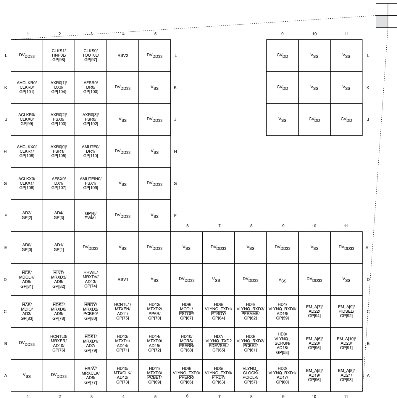
Figure 2-9. GDU Pin Map [Quadrant D]
