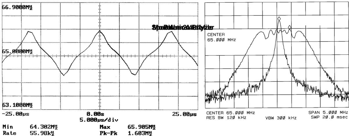
Figure 2. SSCG Clock, SM560, Fin = 65 MHz
