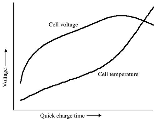
Figure 9. Battery temperature change
