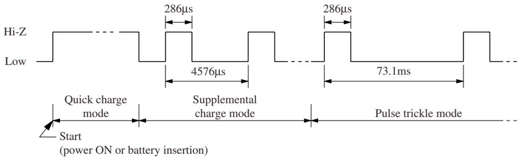
Figure 1. CHGN output (external charger control)
