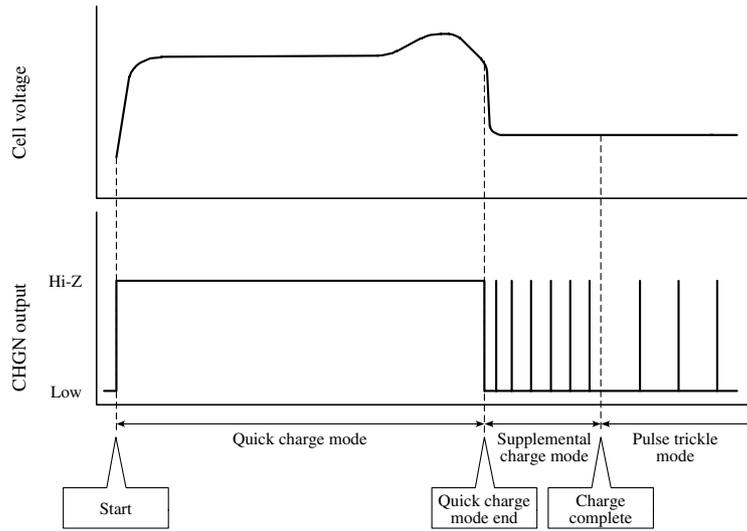
Figure 6. Charging mode, battery voltage and charging current
