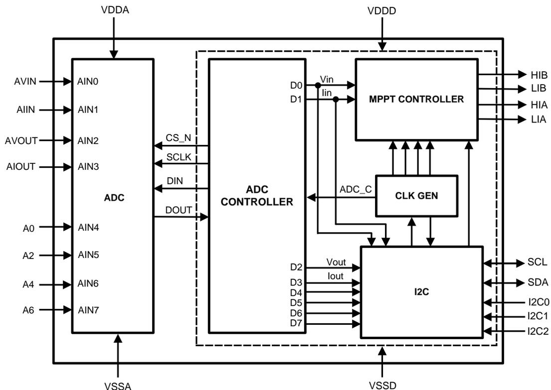
Figure 1. Block Diagram
