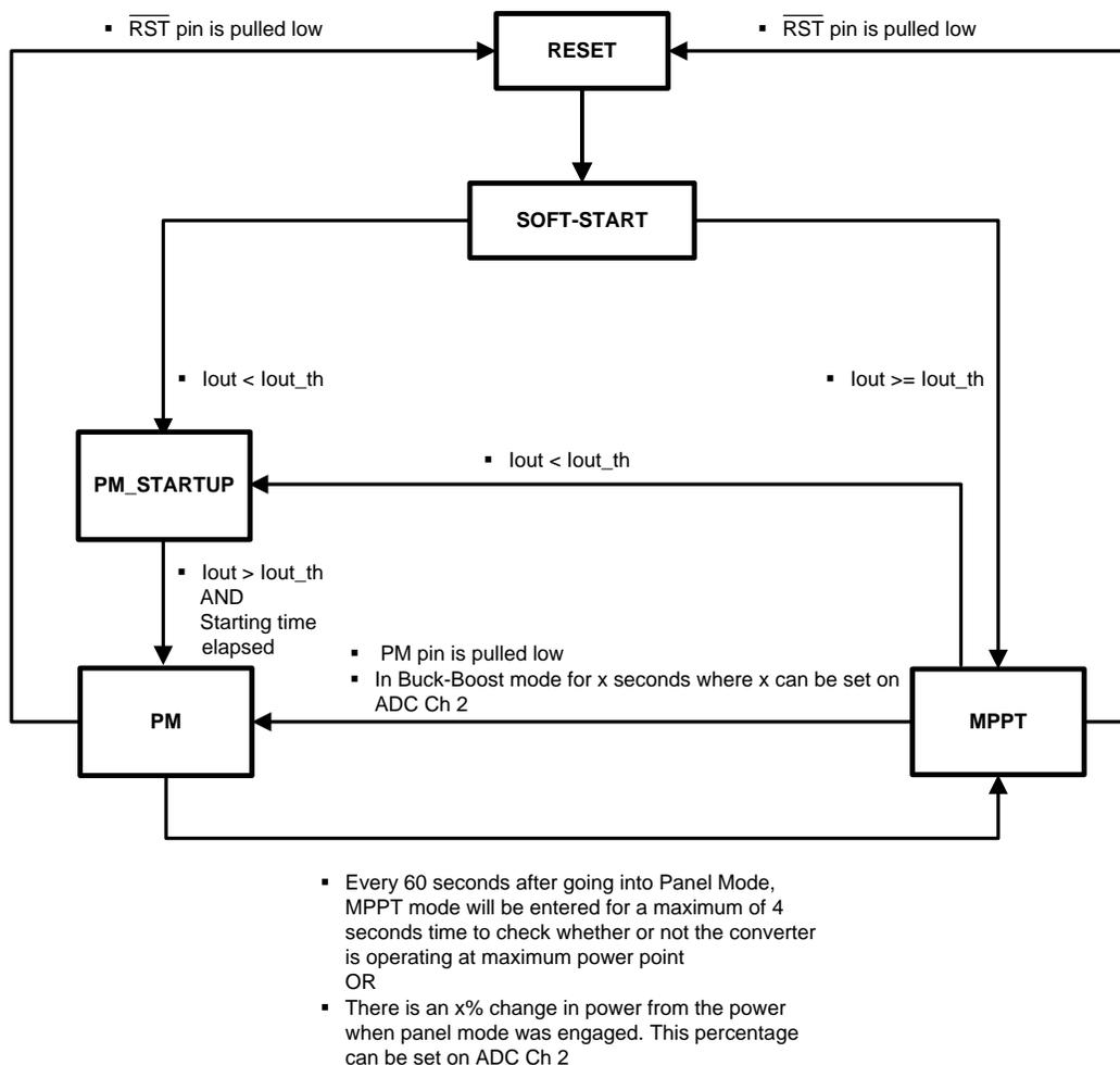
**Figure 4. High Level State Diagram for Startup**
