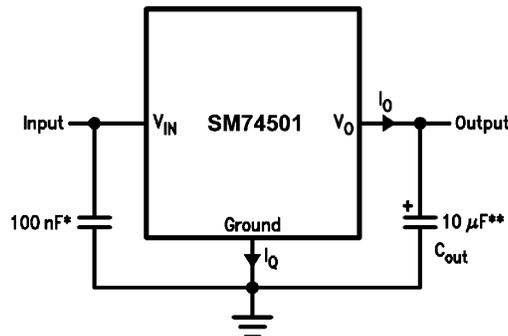
\* Required if regulator is located more than 2 inches from power supply filter capacitor.
