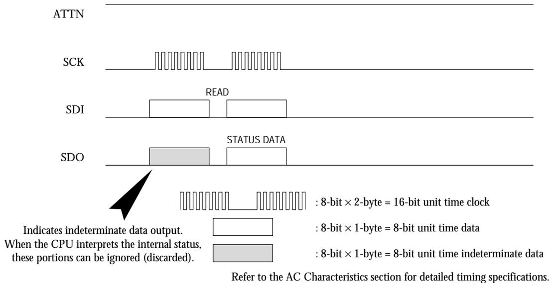
Figure 11. Internal status transfer timing
