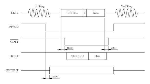
PDWN is an internal signal (set by S0, S1, MODE)
