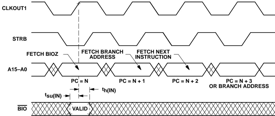
Figure 10.  $\overline{BIO}$  Timing
