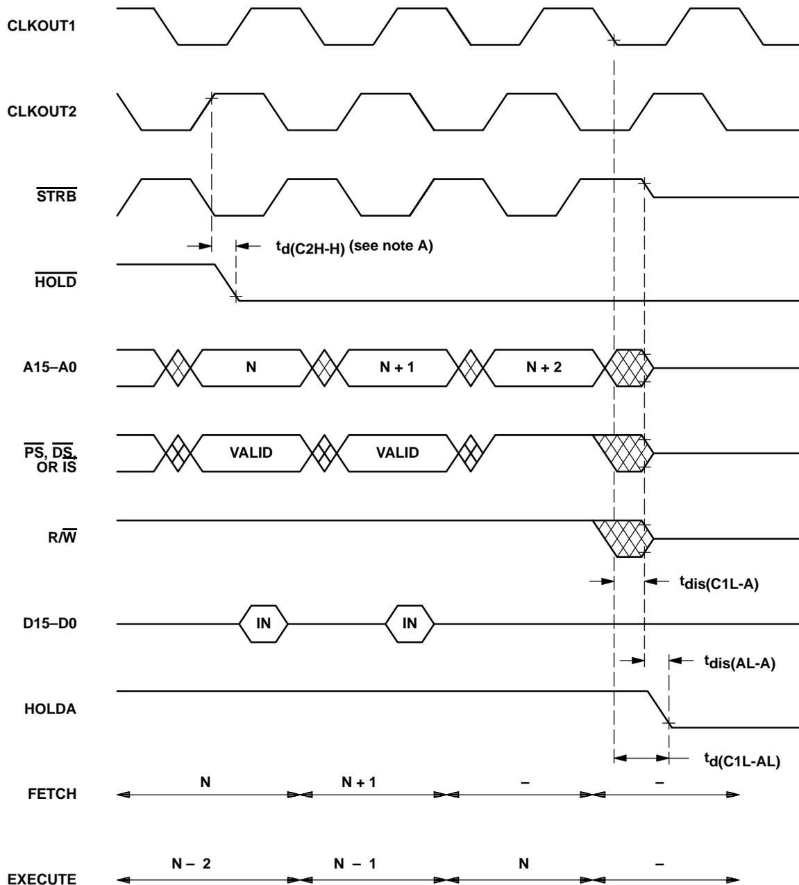
NOTE A:  $\overline{HOLD}$  is an asynchronous input that can occur at any time during a clock cycle. If the specified timing is met, the exact sequence shown will occur; otherwise, a delay of one CLKOUT2 cycle will occur.
