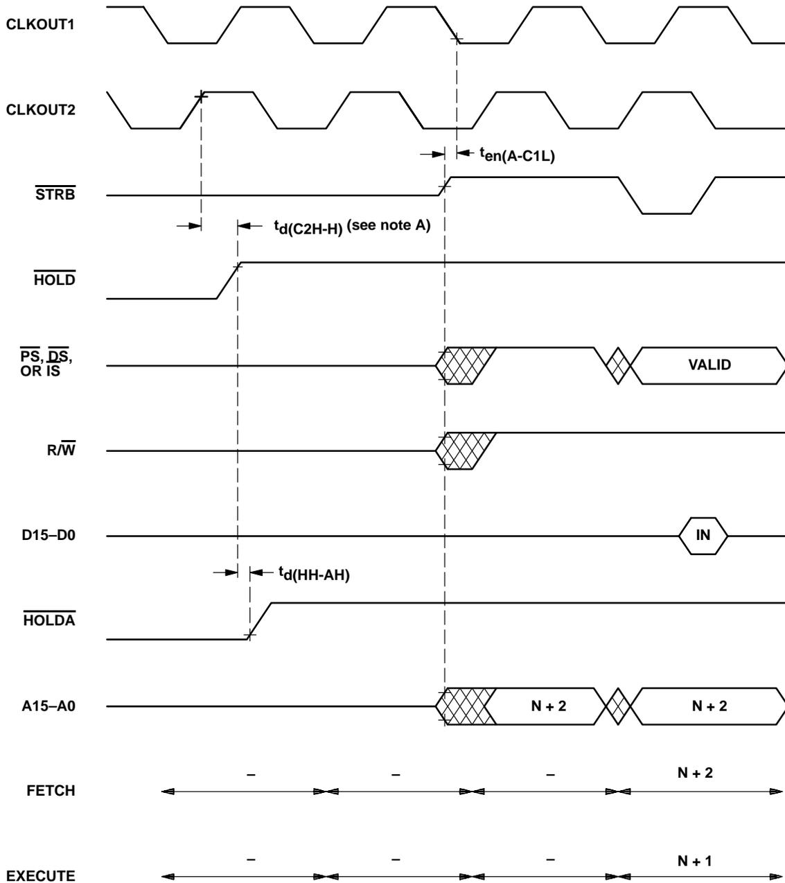
NOTE A:  $\overline{\text{HOLD}}$  is an asynchronous input that can occur at any time during a clock cycle. If the specified timing is met, the exact sequence shown will occur; otherwise, a delay of one CLKOUT2 cycle will occur.
